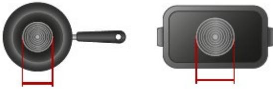
5. If the ferromagnetic part covers only partially the base of the pan, only the ferromagnetic area will heat up, the rest of the base may not heat up a sufficient temperature for cooking.
