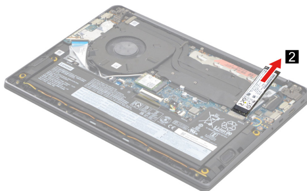
Figure 7. Remove the SSD by pulling it away from the slot
