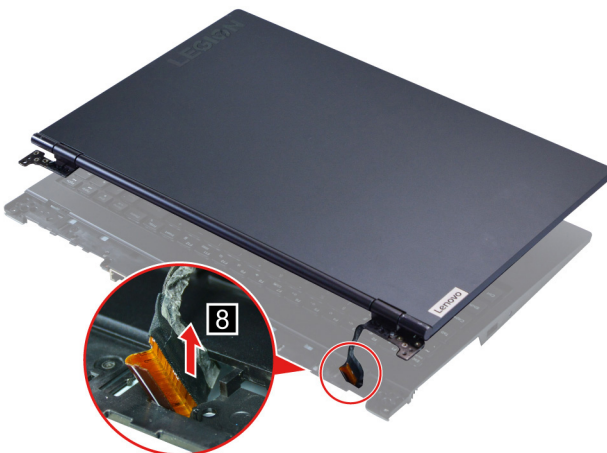
Figure 30. Remove the LCD module
