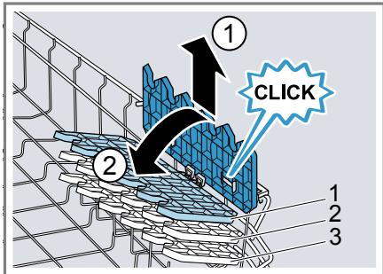
2. Position the etagere at a slight angle and move to the right height ②.
