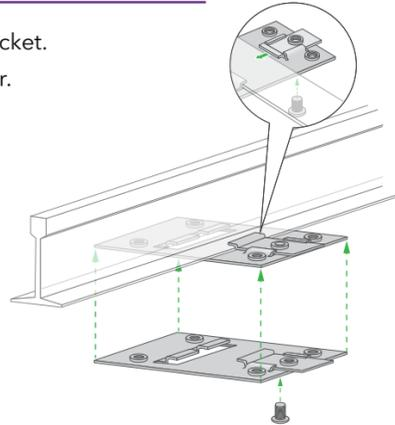
5. Use the four short screws to attach the mounting plate to the T-bar.
