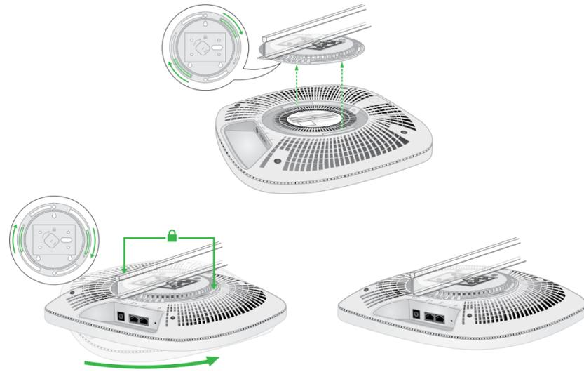
8. Twist the access point clockwise to lock it onto the mounting plate.
