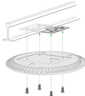
7. Hold the access point upside down and attach it to the mounting plate.
