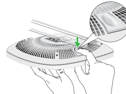
3. Turn the access point counterclockwise until the access point releases from the mounting plate.
