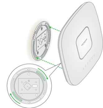
5. Twist the access point clockwise to lock it onto the mounting plate.
