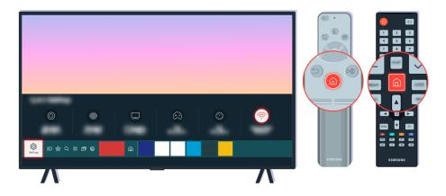
If your TV is connected to the Internet, you can set it to receive periodic updates automatically. On the remote control, press the figure button and move to 🕸 Settings using the directional button.
