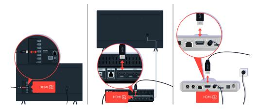
Check the antenna and HDMI cable connections.
