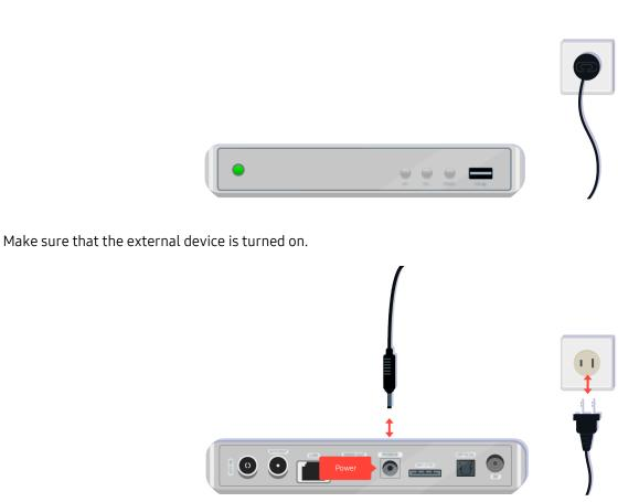
If it does not turn on, make sure the power cable is properly connected to the device and to the wall outlet.
