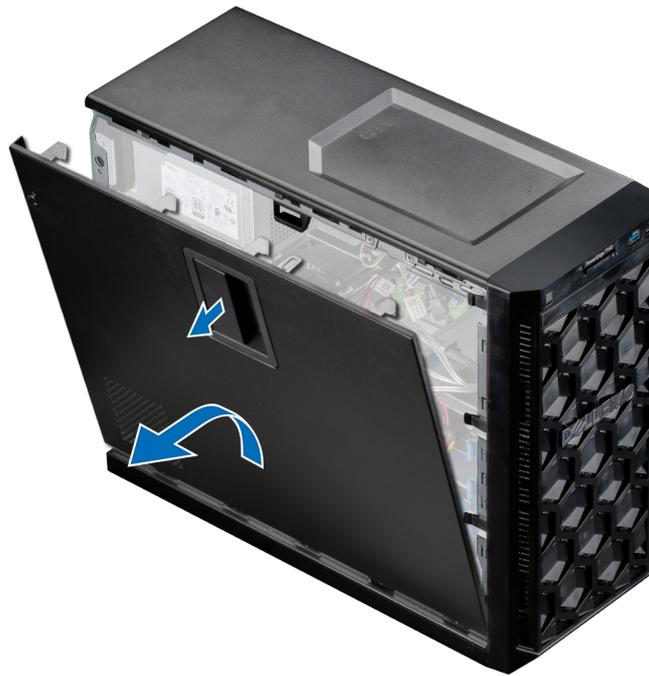
**Figure 9. Removing the system cover**
