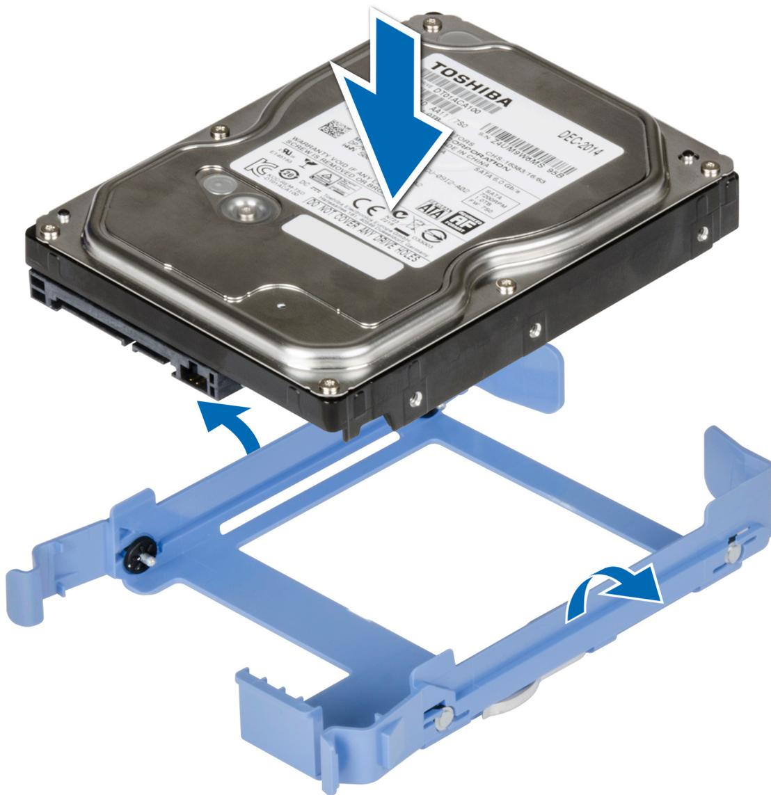
Figure 16. Installing a drive into the drive carrier
