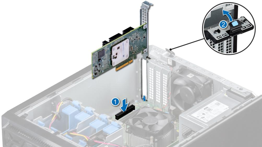
**Figure 33. Installing an integrated storage controller card**
