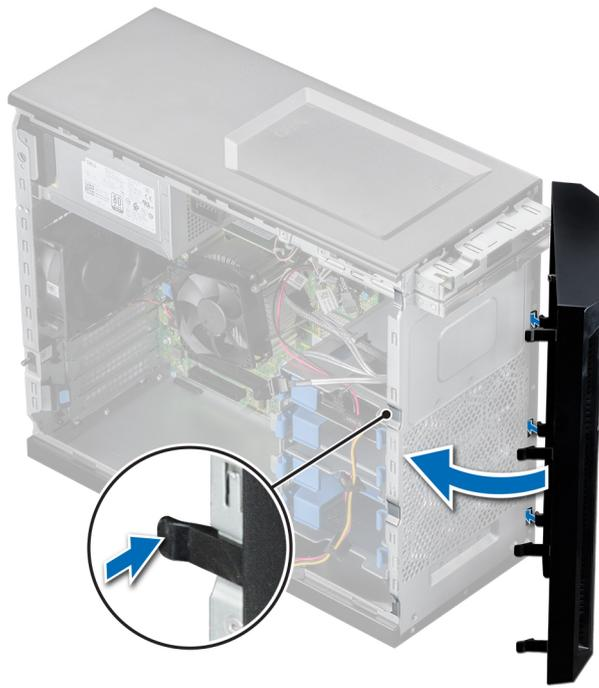
Figure 12. Installing the front bezel
