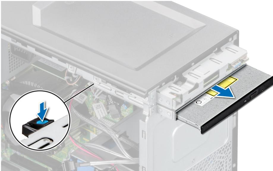
**Figure 21. Removing the optical drive**
