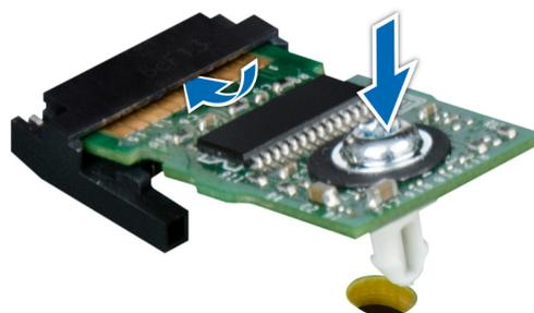
Figure 53. Installing the TPM
