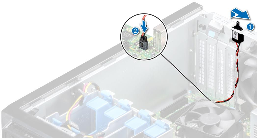
**Figure 49. Installing the intrusion switch**
