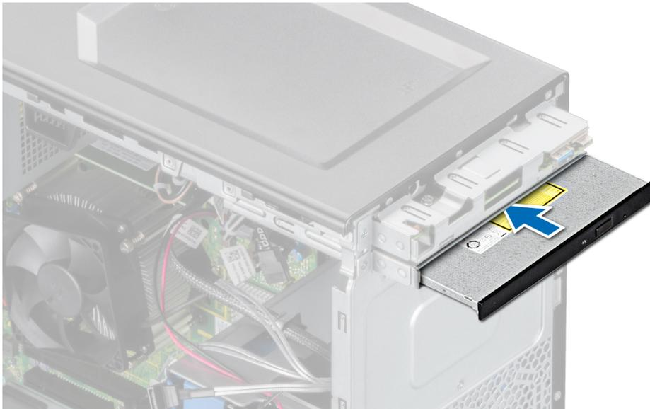
**Figure 22. Installing the optical drive**
