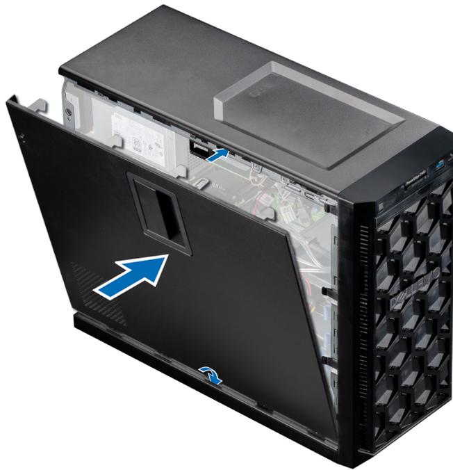
Figure 10. Installing the system cover
