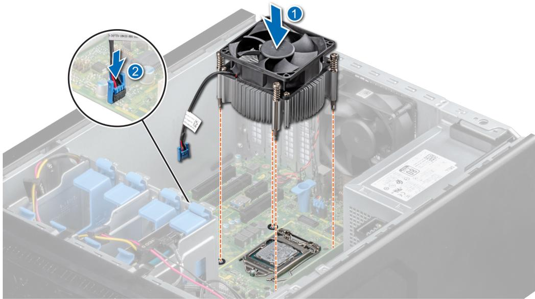
**Figure 42. Installing the heat sink**
