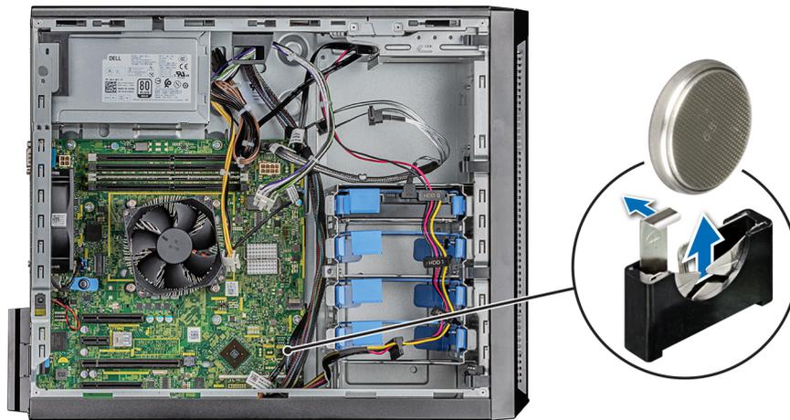
**Figure 46. Removing system battery**
