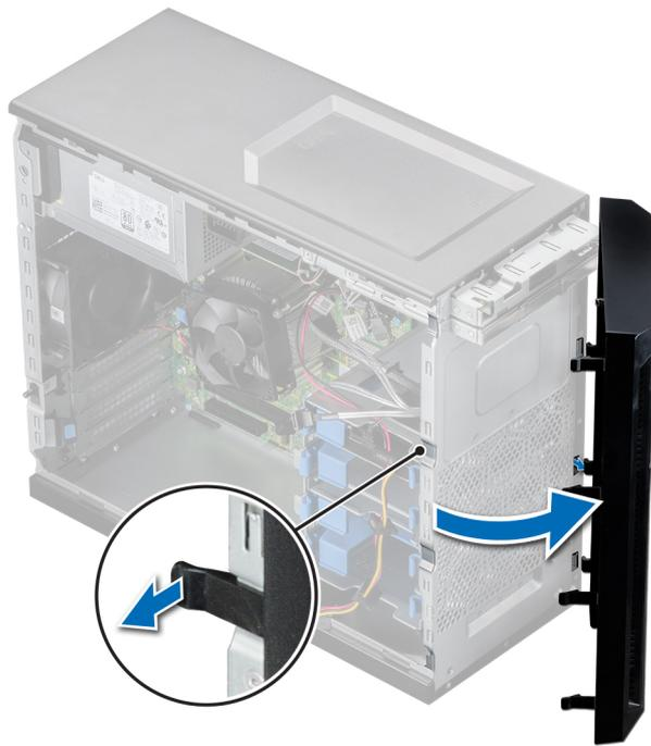
**Figure 11. Removing the front bezel**
