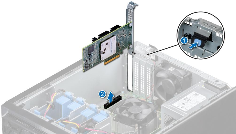
**Figure 32. Removing the integrated storage controller card**
