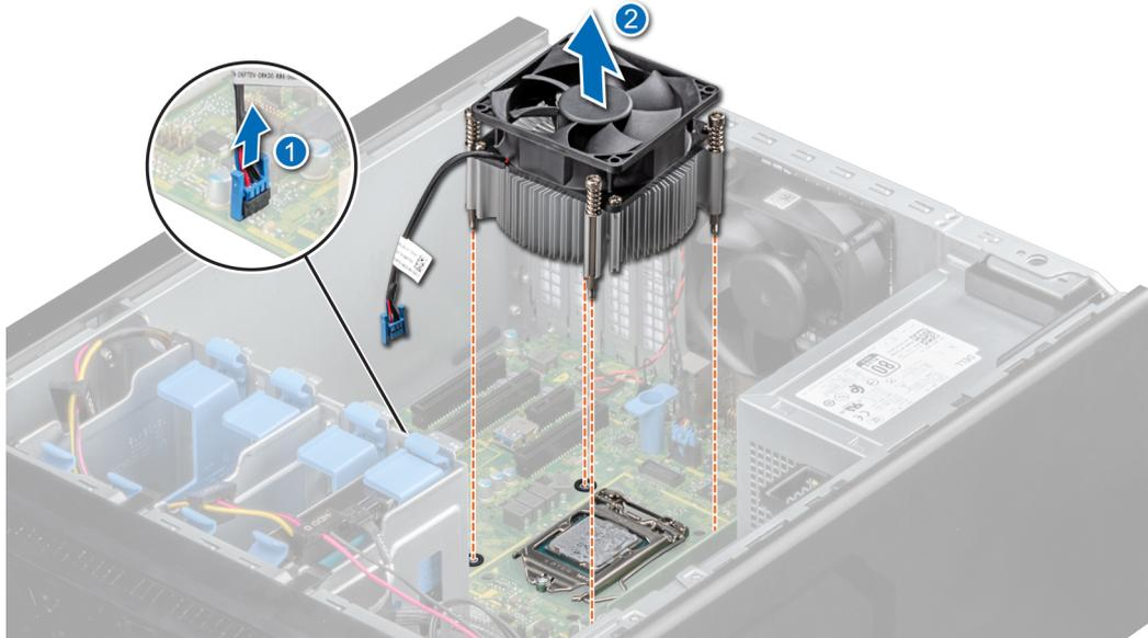
Figure 38. Removing the heat sink
