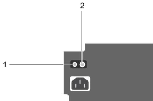
**Figure 62. Non-redundant cabled AC PSU status indicator and self-diagnostic button**
