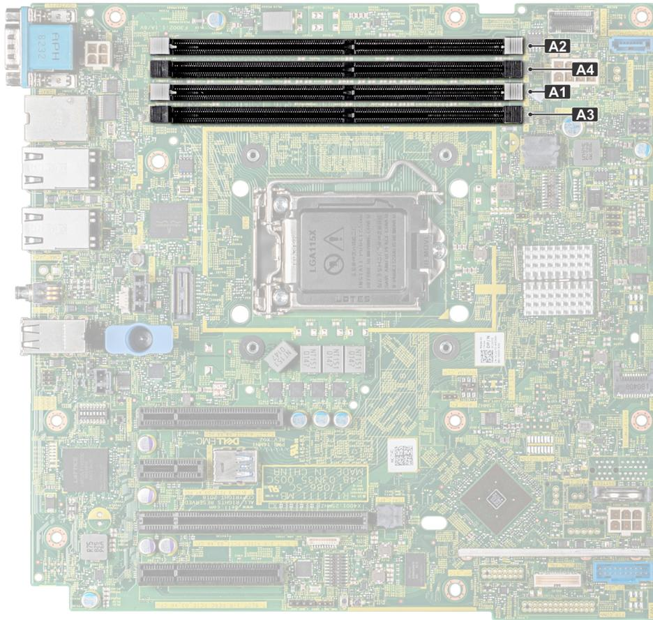
**Figure 23. Memory socket locations on the system board**
