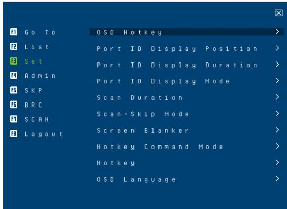
Clicking **F3 Set** or pressing **F3** activates the Set function. This function allows the administrator and each user to set up his own working environment. A separate profile for each is stored by the OSD and is activated according to the username that was provided during login.
