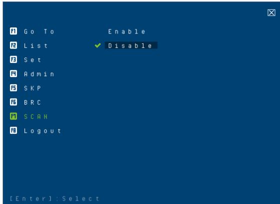
Clicking **F7 SCAN** or pressing **[F7]** invokes *Auto Scan* mode. This function allows you to automatically switch among the available computers at regular intervals so that you can monitor their activity without having to take the trouble of switching yourself. Enable mouse emulation for *Auto Scan* to work (see page 42).
