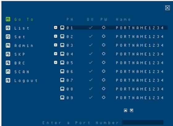
Clicking **F1 G O T O** or pressing **[F1]** activates the Go To function. Go To allows you to switch directly to a port by keying in the port's ID. Enable mouse emulation for independent switching (see page 42), for this function to work.
