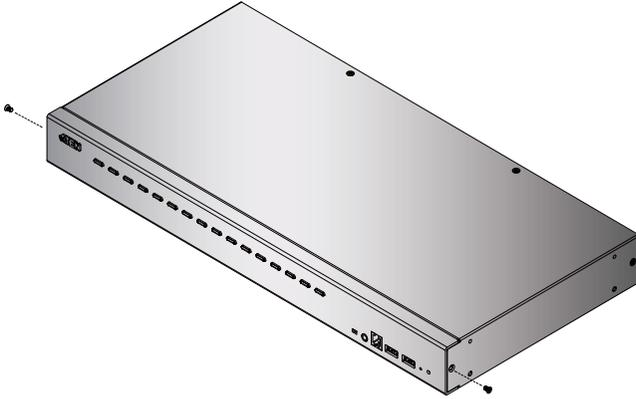
2. Use the M3 x 6 Phillips hex head screws supplied with the rack mounting kit to screw the rack mounting brackets into the sides near the front of the unit.
