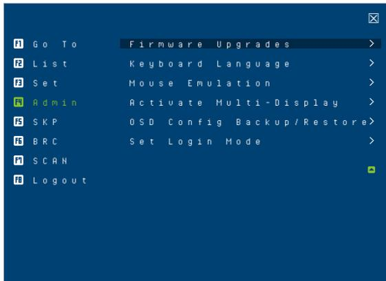
Clicking **[F4] Admin** or pressing **[F4]** activates Admin function. F4 is an administrator only function. It allows the administrator to configure and control the overall operation of the OSD. To change a setting, click on the settings item you want to configure, or use the up and down arrow keys to move the highlight bar to it then press **[Enter]**.
