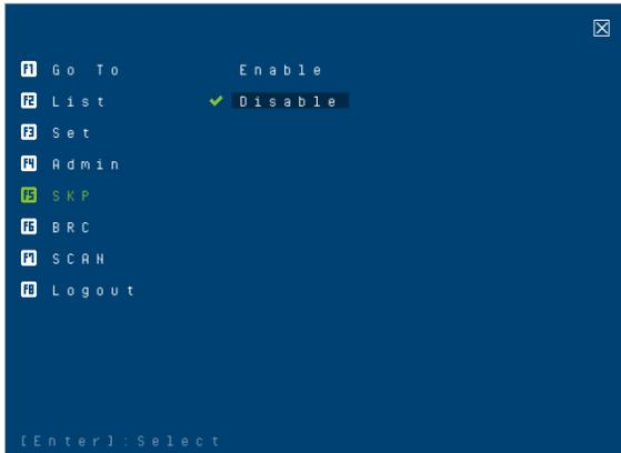
Clicking **F5 SKP** or pressing **[F5]** invokes Skip (SKP) mode. This function enables you to easily skip backward or forward – switching the console focus from the currently active computer port to the previous or next accessible one. Enable mouse emulation for Skip mode to work (see page 42).
