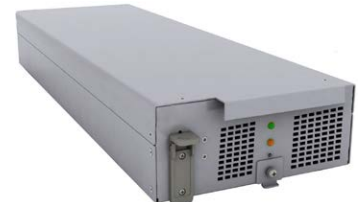
Liebert® APS Charger Module 10A battery charger that operates in parallel with the chargers integrated in each Power module. To increase runtime in the Liebert APS, this 10A charger should be used when battery string to power module ratio is greater than 3:1.
