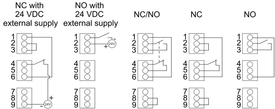
The EPO input supports 24 VDC.
