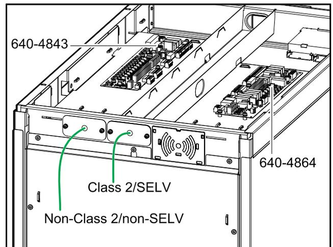
15. Route the non-Class 2/non-SELV signal cables through the left rear brush/ gland plate and into the left side of the UPS.
