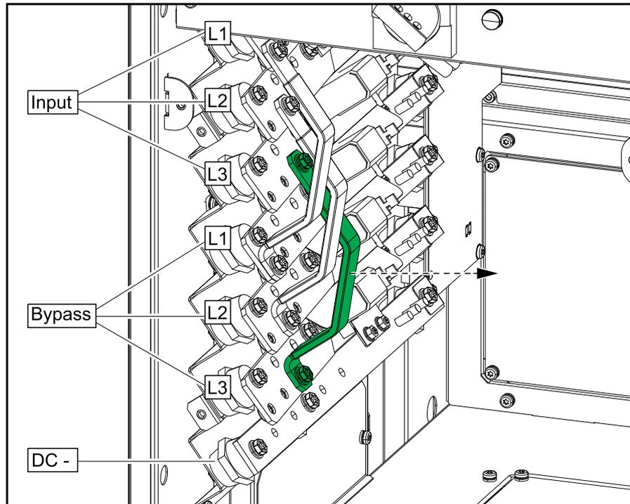
3. Install the NEMA 2 hole plates and connect the power cables as shown in the described order:
