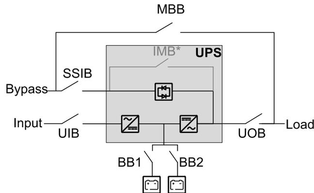
**NOTE:** The internal maintenance breaker IMB\* cannot be used in a system with an external maintenance bypass breaker MBB and the internal maintenance breaker IMB\* must be padlocked in the open position.
