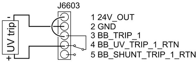
**Battery Breaker Trip Connection with External 24 VDC Supply**
