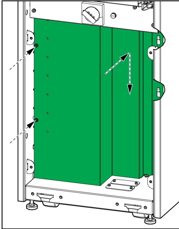
4. Reinstall the lower front plate.
