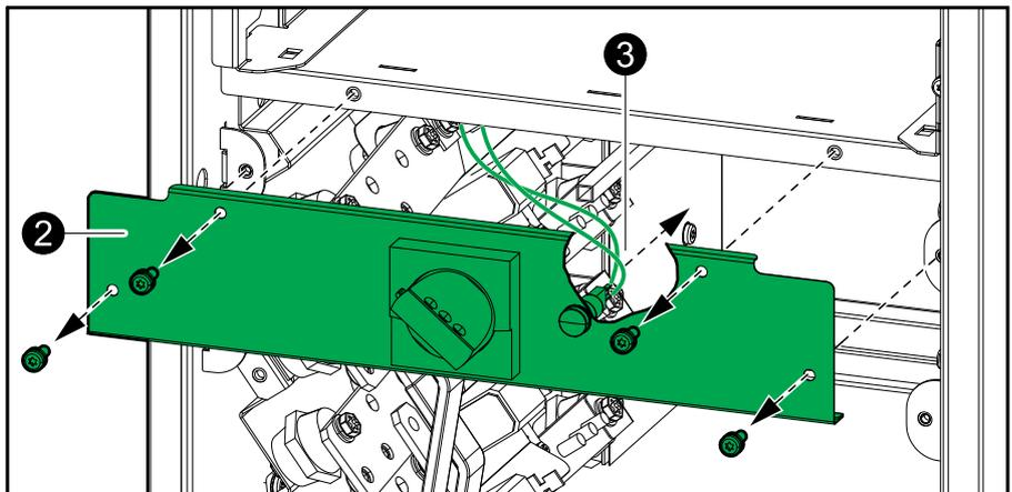
3. Disconnect the signal cables from the internal maintenance breaker IMB indicator light on both UPSs.
