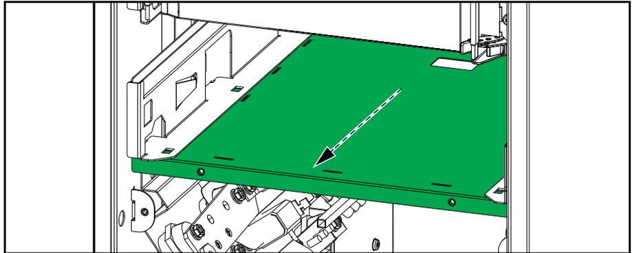
5. Remove the front cover from the internal maintenance breaker IMB on both UPSs.
