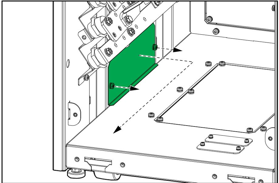
7. **For installation with maintenance bypass cabinet:** Remove the right side panel. The side panel will be reinstalled on the maintenance bypass cabinet.
