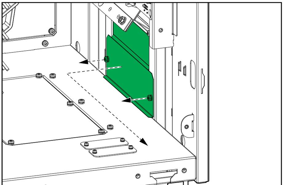
9. **For bottom cable entry:** Remove the gland plate in the bottom of the UPS.
