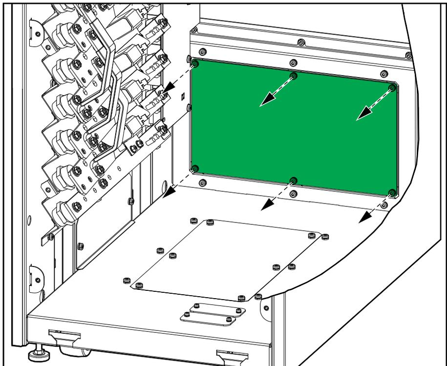
11. Drill/punch holes for power cables/conduits in the gland plate. Install conduits (not provided), if applicable.
