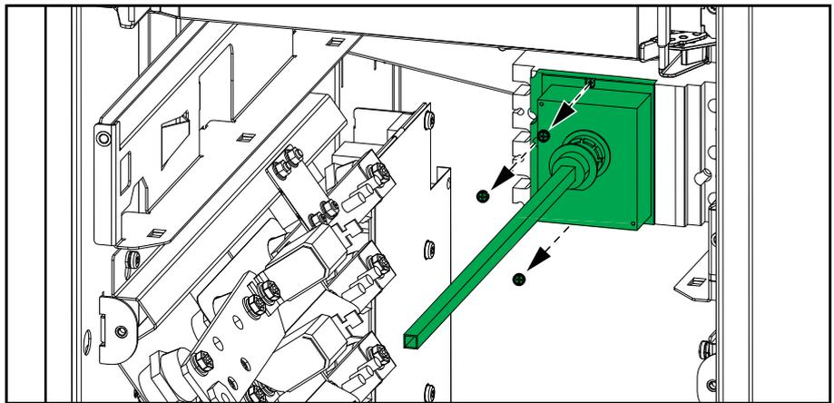
6. Install an additional AUX switch (provided) in the OF2 position in the internal maintenance breaker IMB on both UPSs.
