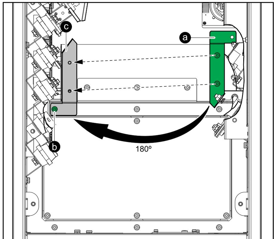
2. **Only for dual mains system:** Remove the three single mains jumper busbars.
