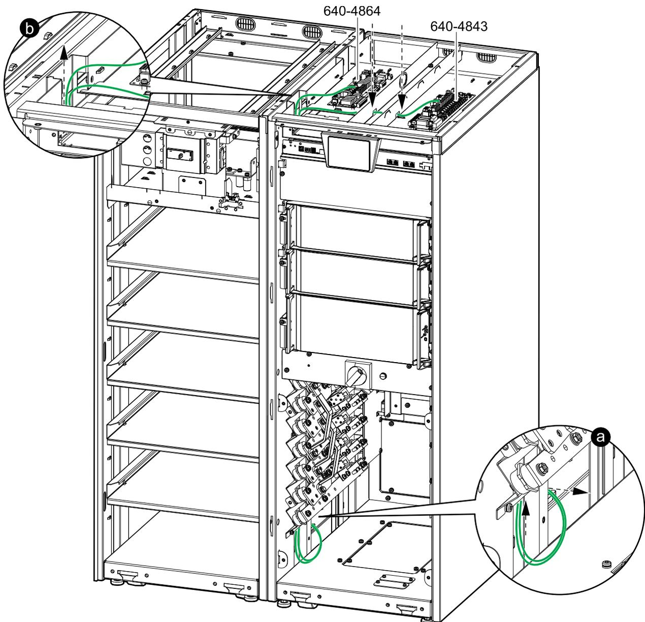
3. Connect the signal cables from modular battery cabinet 1 to the UPS:
