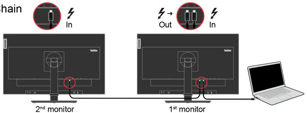
11. Connect Intel vPro<sup>®</sup> supported Notebook through P27u-20 Thunderbolt™ 4 interface can let you remotely access/control computer via Intel Active Management Technology (Intel<sup>®</sup> AMT) when the operating system is not available or even the computer is turned off.
