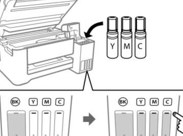
**8** When the ink reaches the upper line of the tank, pull out the bottle.
