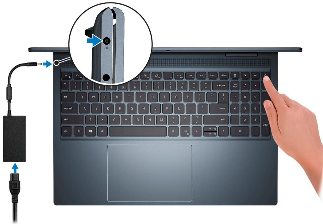
***(i)* NOTE:** The battery may go into power-saving mode during shipment to conserve charge on the battery. Ensure that the power adapter is connected to your computer when it is turned on for the first time.
