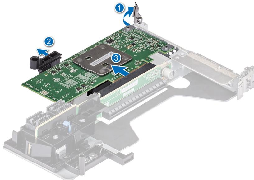
Figure 6. Remove the Dell HBA355i Adapter
