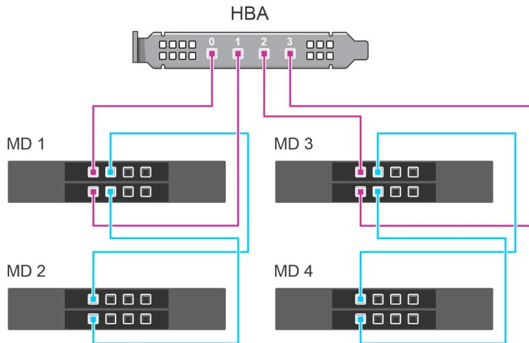
**Figure 14. Multipath Configuration: Cabling HBA355e Adapter with MD1420 and MD1400 Enclosures**
