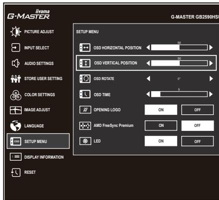
Press the ENTER Button and finally the EXIT Button to close the On Screen Display feature. All changes are saved in the memory.
