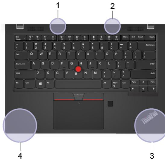
1. Antenna WLAN (wireless LAN) (ausiliaria)
