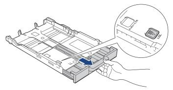
4. Gently press and slide the paper width guides (1) and the paper length guide (2) to fit the paper size.
