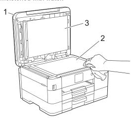
3. In the ADF unit, clean the white bar (1) and the glass strip (2) with a lint-free cloth moistened with water.
