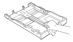
6. Wipe the outside of the paper support with a dry, lint-free cloth to remove dust.
