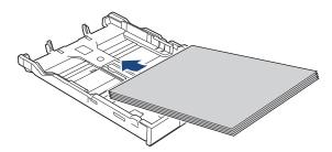
Make sure the paper is flat in the tray and the paper length guide (1) touches the edges of the paper.
