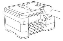
5. Wipe the inside and the outside of the paper tray with a dry, lint-free cloth to remove dust.
