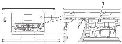
6. Lift the flap (2), and then clean the back side of the Paper Feed Rollers (1) with a soft lint-free cloth moistened with water. After cleaning, wipe the rollers with a dry, soft lint-free cloth to remove all moisture.
