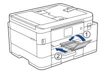
2. Pull the paper tray completely out of the machine.
