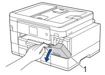
2. Press the lock release lever to release the ink cartridge color indicated on the LCD and remove the ink cartridge from the machine, as shown in the illustration.
