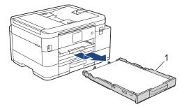
3. Lift the paper support (1), and then pull it at an angle completely out of the machine as shown by the arrow.
