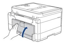
5. Put the paper support firmly back in the machine. Make sure you fit the paper support into the channels.
