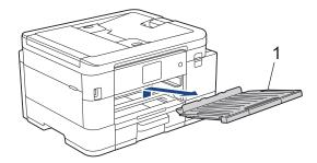
5. Clean the Paper Pick-up Rollers (1) with a soft lint-free cloth moistened with water. Slowly turn the rollers so that the whole surface is cleaned. After cleaning, wipe the rollers with a dry, soft lint-free cloth to remove all moisture.
