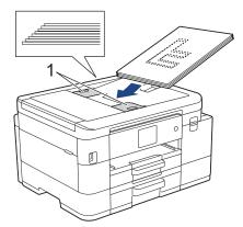
4. Place your document, **face down**, **top edge first** in the ADF underneath the paper guides until you feel the document touch the feed rollers and the LCD displays [ADF Ready].
