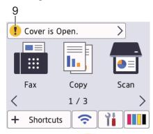
The warning icon papears when there is an error or maintenance message; press to view the details, and then press to return to the Home screen.
