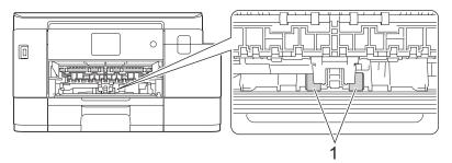
6. Put the paper support firmly back in the machine. Make sure you fit the paper support into the channels.
