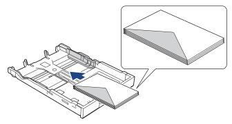
4. Gently press and slide the paper width guides (1) and paper length guide (2) to fit the size of the envelopes. Make sure the envelopes are flat in the tray.
