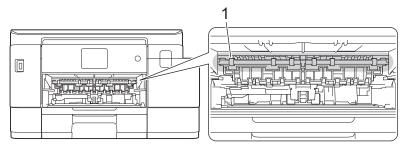
b. (MFC-J4335DW/MFC-J4345DW) Squeeze both levers (1), and then open the Jam Clear Cover at the back of the machine.
