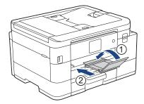
2. Pull the paper tray completely out of the machine.
