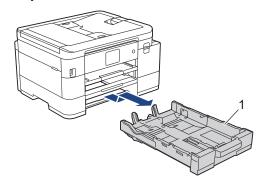
3. Lift the paper support (1), and then pull it at an angle completely out of the machine as shown by the arrow.
