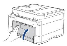
7. If your LCD error message was [Jam Rear], put the paper support firmly back in the machine. Make sure you fit the paper support into the channels.
