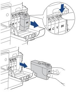
3. Open the new ink cartridge bag for the color indicated on the LCD, and take out the ink cartridge.
