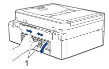
(MFC-J4535DW) Open the Jam Clear Cover (1) on the back of the machine.
