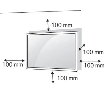
To install your monitor on a wall, attach a wall mounting bracket (optional part) to the back of the monitor. Make sure that the wall mounting bracket is securely fixed to the monitor and to the wall.
