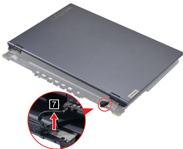
Figure 34. Take out the EDP cable and then remove the LCD module
