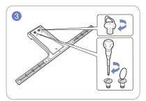
Tightly fasten the connecting screw at the bottom of the stand base.
