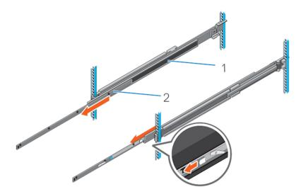
Figure 26. Pull out the intermediate rail
