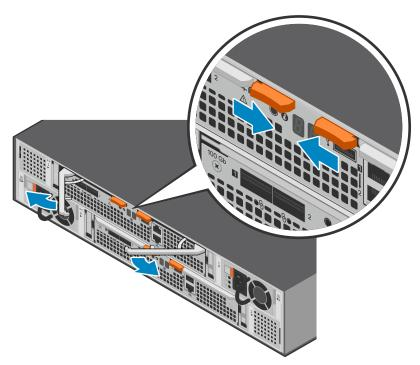
Figure 129. Releasing the Access Module
