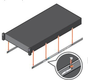
Figure 27. Attach the inner rails to the system
