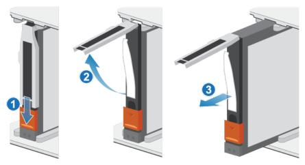
Figure 101. Removing a drive
