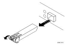
Figure 62. Removing an SFP module
