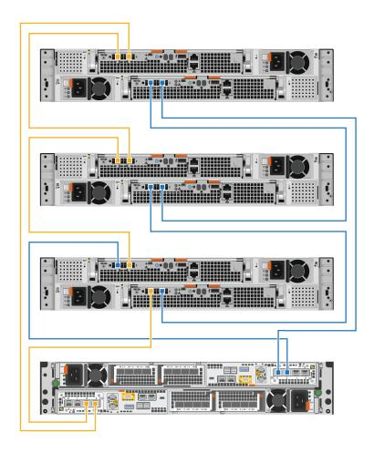
Figure 19. Cabling three expansion enclosures
