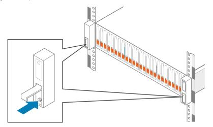
Figure 4. Tightening the captive screws
