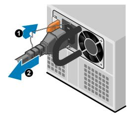
Figure 109. Removing the power cable
