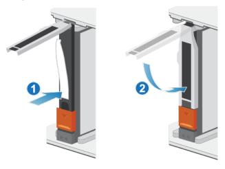
Figure 102. Installing a drive
