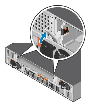
Figure 128. Locking the DIB into place
