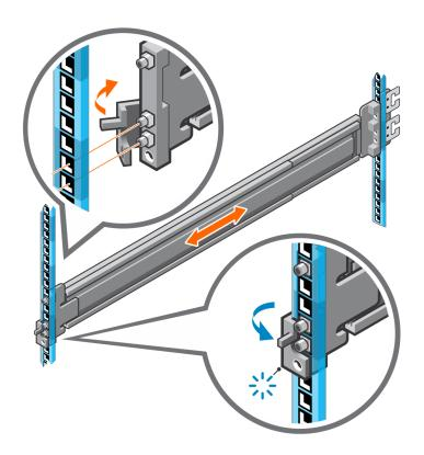
Figure 10. Installing the NVMe expansion enclosure rails (front)
