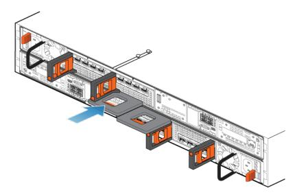
Figure 78. Installing the node
