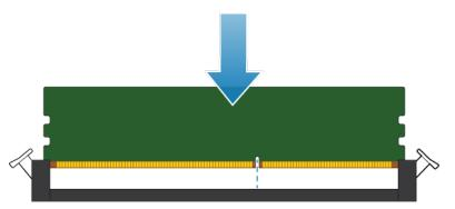
Figure 85. Installing the DIMM
