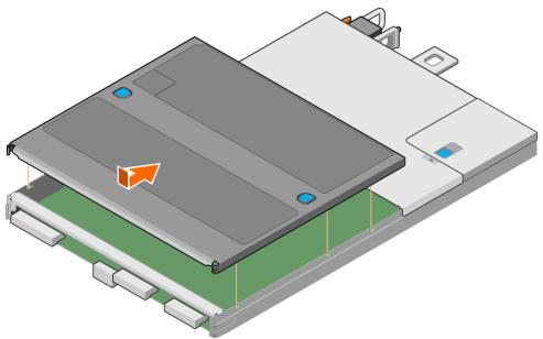
Figure 97. Installing the top cover
