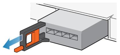
Figure 66. Removing the I/O module
