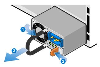
Figure 47. Removing a DC power supply
