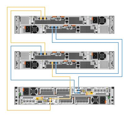
Figure 31. Cabling two expansion enclosures
