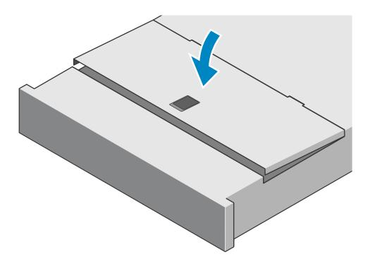
Figure 120. Closing the system cover
