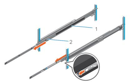
Figure 12. Pull out the intermediate rail
