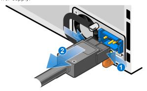
Figure 46. Removing a DC power cable
