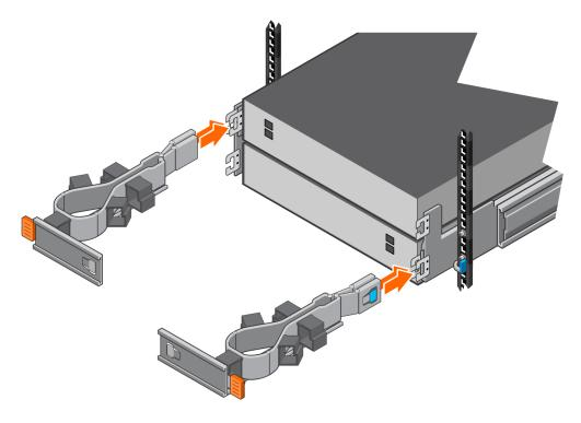
Figure 30. Installing the cable management arms
