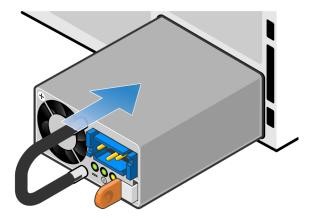
Figure 48. Installing a DC power supply
