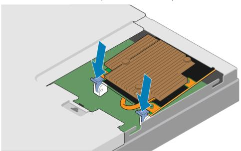
Figure 55. Opening the retaining tabs
