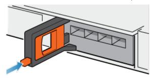
Figure 68. Locking the I/O module into place
