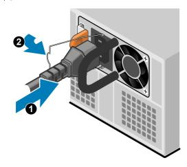
Figure 112. Inserting the power cable
