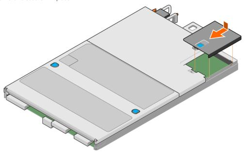
Figure 59. Installing the embedded module cover
