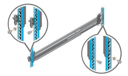
Figure 11. Adding the retaining screws
