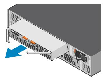
Figure 130. Removing the Access Module
