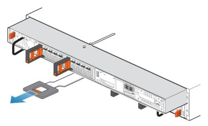
Figure 91. Removing the node
