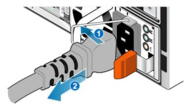
Figure 41. Removing the power cable
