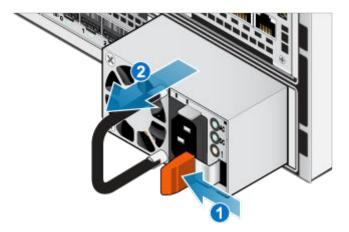
Figure 42. Removing a power supply
