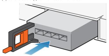
Figure 67. Installing an I/O module
