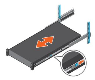
Figure 29. Slide system into the rack
