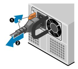
Figure 110. Removing a power supply
