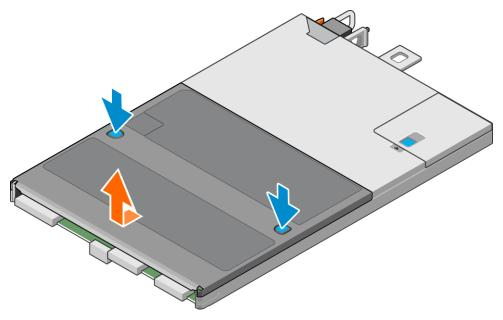
Figure 72. Removing the top cover
