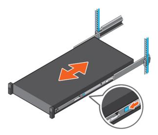
Figure 15. Slide system into the rack
