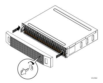
Figure 35. Installing the bezel
