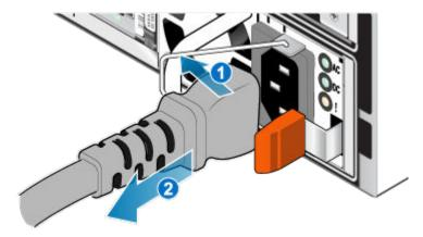
Figure 51. Removing the power cable
