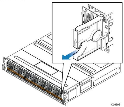
Figure 105. Removing a drive filler module
