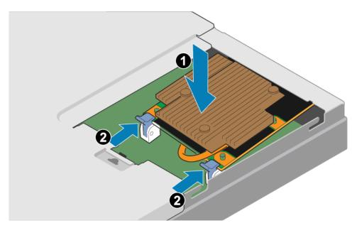
Figure 58. Locking the 4-port card into position
