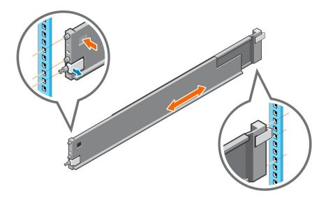
Figure 1. Installing the rails
