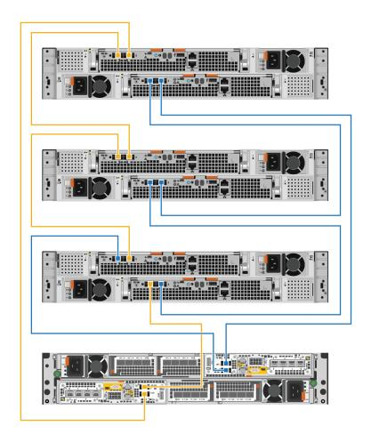
Figure 32. Cabling three expansion enclosures
