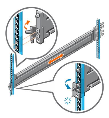
Figure 24. Installing the NVMe expansion enclosure rails (front)
