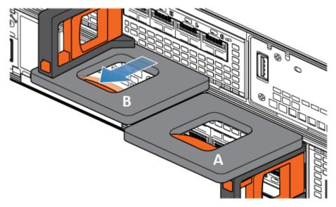
Figure 80. Disengaging the locking mechanism for node B
