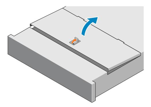
Figure 113. Lifting the system cover
