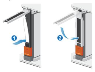
Figure 34. Installing a drive
