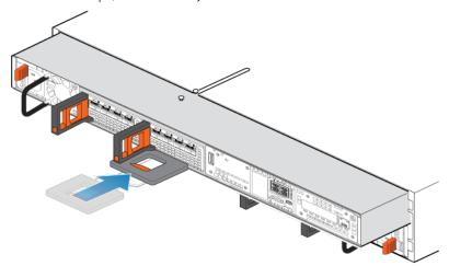
Figure 77. Sliding the node halfway into the chassis
