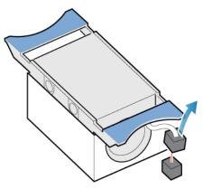
Figure 73. Disconnecting the fan power cable
