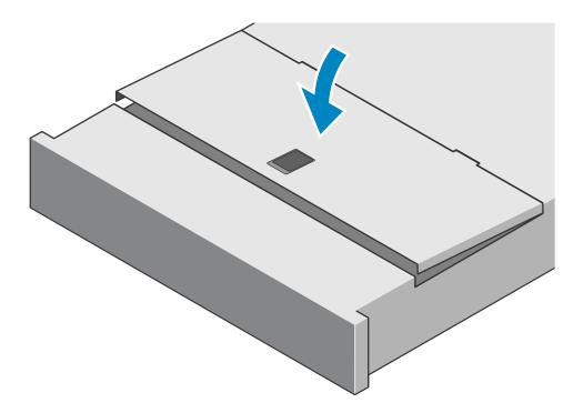
Figure 116. Closing the system cover
