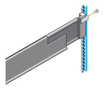
Figure 2. Installing the security screws
