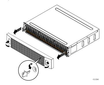
Figure 100. Removing the front bezel
