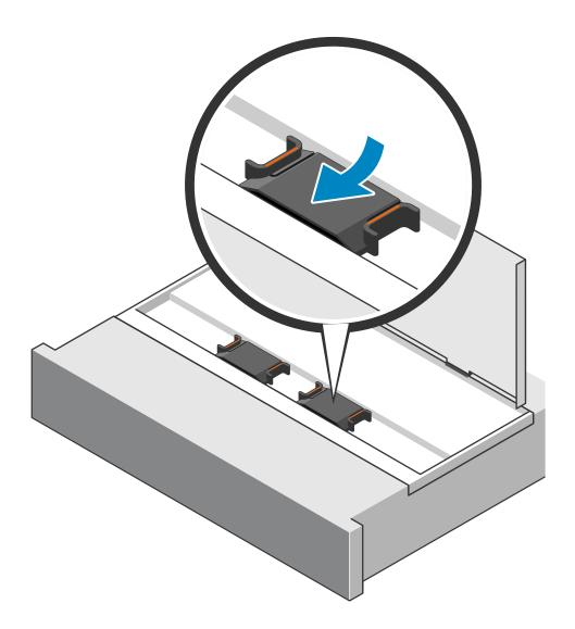
Figure 119. Installing the Clock Distribution Board
