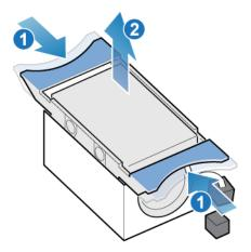
Figure 74. Removing the fan from the motherboard
