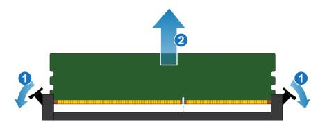
Figure 132. Removing the DIMM
