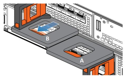
Figure 52. Disengaging the locking mechanism for node B
