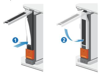
Figure 21. Installing a drive
