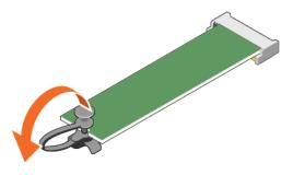
Figure 93. Releasing the internal M.2 boot module from the motherboard
