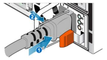
Figure 44. Inserting the power cable
