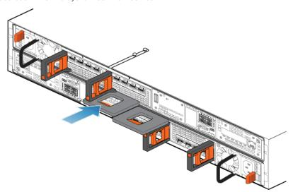
Figure 61. Installing the node
