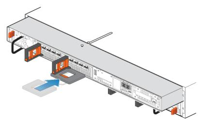
Figure 98. Sliding the node halfway into the chassis
