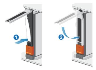
Figure 39. Installing a 2.5" drive
