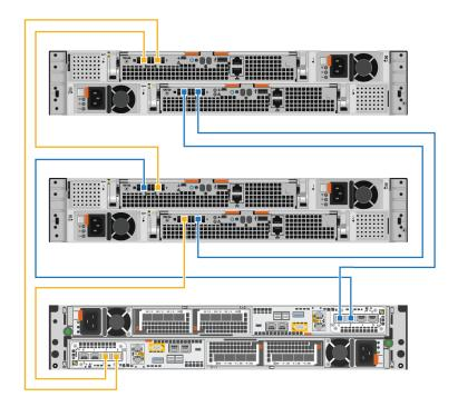
Figure 18. Cabling two expansion enclosures
