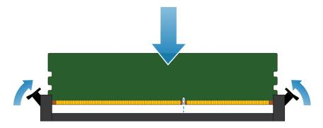
Figure 133. Installing the DIMM
