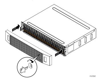
Figure 103. Installing the bezel
