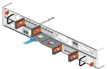
Figure 99. Installing the node
