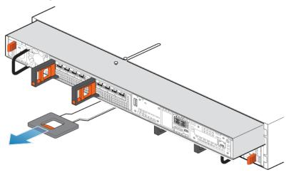
Figure 71. Removing the node
