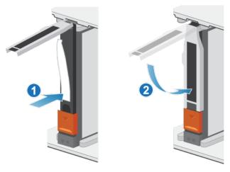
Figure 106. Installing a drive
