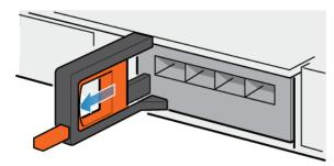
Figure 65. Releasing the I/O module
