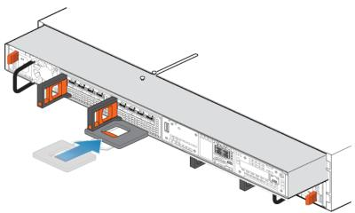
Figure 87. Sliding the node halfway into the chassis
