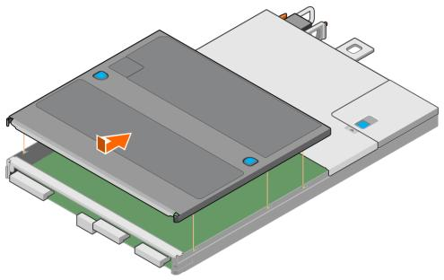
Figure 86. Installing the top cover
