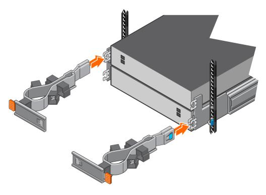
Figure 16. Installing the cable management arms
