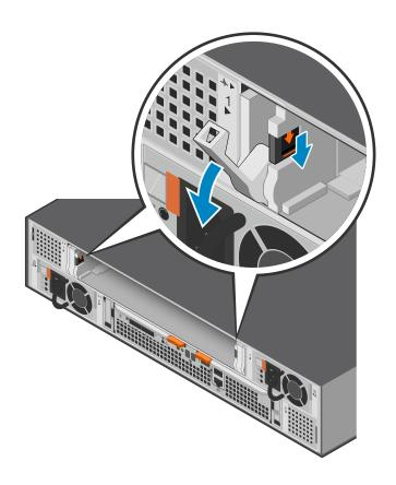
Figure 125. Releasing the DIB
