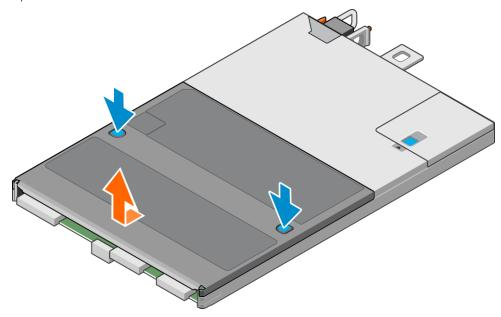
Figure 92. Removing the top cover
