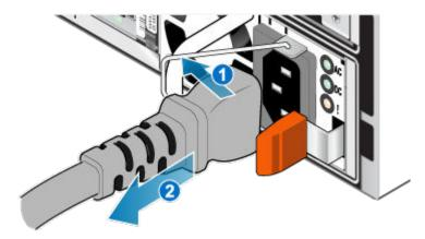
Figure 79. Removing the power cable
