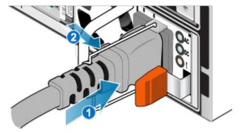
Figure 5. Inserting the power cable
