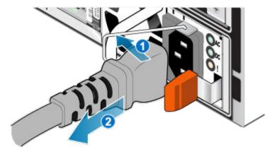
Figure 89. Removing the power cable
