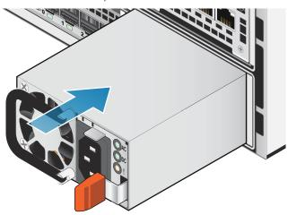
Figure 43. Installing a power supply
