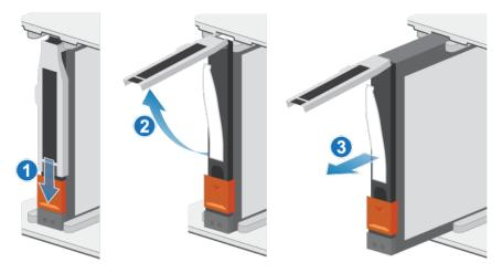
Figure 36. Removing a 2.5" drive
