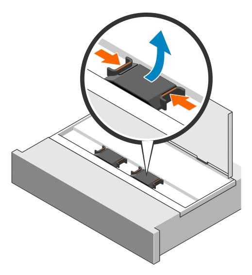
Figure 118. Removing the Clock Distribution Board
