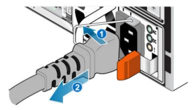
Figure 69. Removing the power cable
