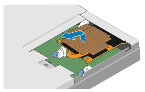
Figure 56. Removing the 4-port card
