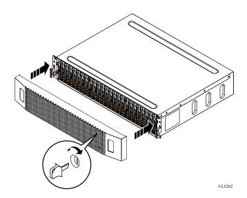
Figure 107. Installing the bezel
