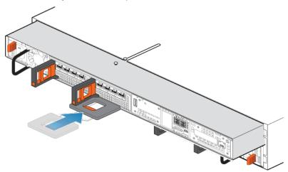
Figure 60. Sliding the node halfway into the chassis
