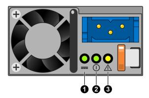
Figure 45. Base enclosure DC power supply LEDs
