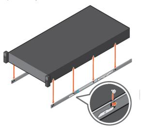
Figure 13. Attach the inner rails to the system
