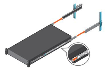
Figure 28. Install system into the extended rails
