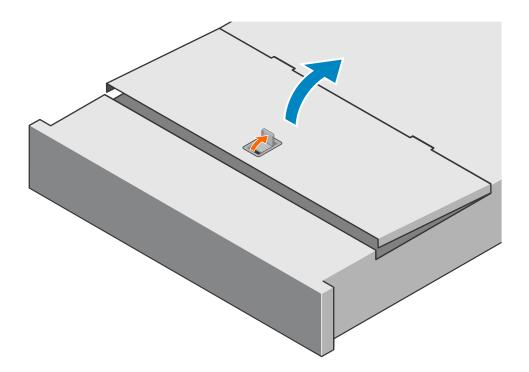
Figure 117. Lifting the system cover
