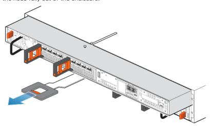
Figure 81. Removing the node
