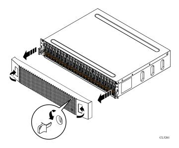
Figure 104. Removing the front bezel
