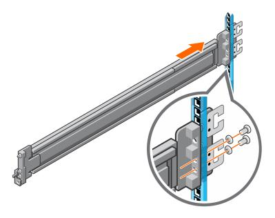
Figure 9. Installing the NVMe expansion enclosure rails (rear)
