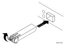
Figure 63. Installing an SFP module
