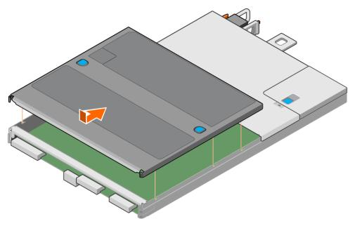
Figure 76. Installing the top cover
