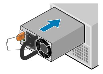
Figure 111. Installing a power supply
