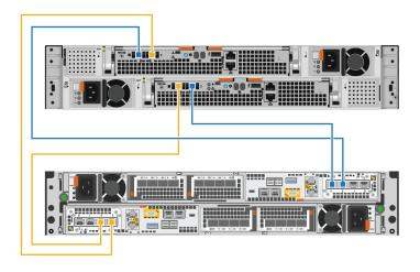
Figure 17. Cabling a single expansion enclosure
