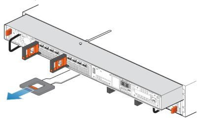
Figure 53. Removing the node
