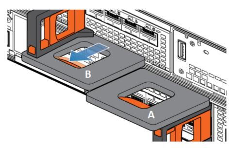
Figure 90. Disengaging the locking mechanism for node B
