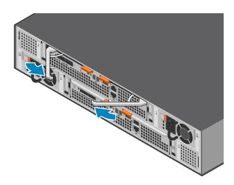
Figure 135. Locking the Access Module into place
