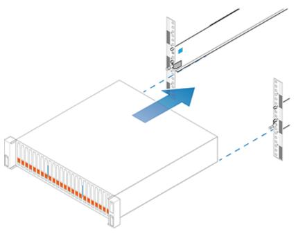
Figure 3. Installing the enclosure
