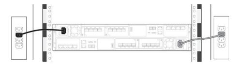
Figure 6. Connecting to the PDU
