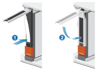
Figure 37. Installing a 2.5" drive
