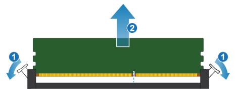
Figure 84. Removing the DIMM
