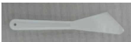
A photograph of a white plastic Hera Jig, a U-shaped tool used for marking straight lines on materials.                                                                                                                                                                                                 |
