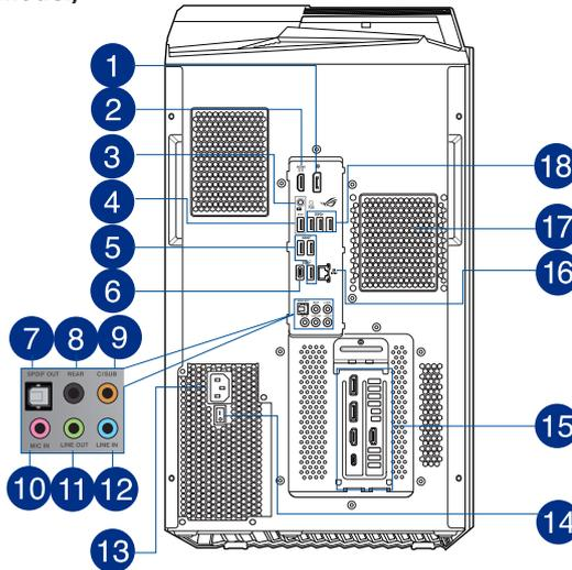
1 **DisplayPort.** This port is for a DisplayPort-compatible device.
