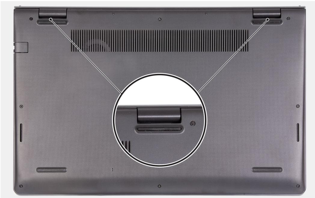
4. Lift and slide the base cover off the palm-rest and keyboard assembly.
