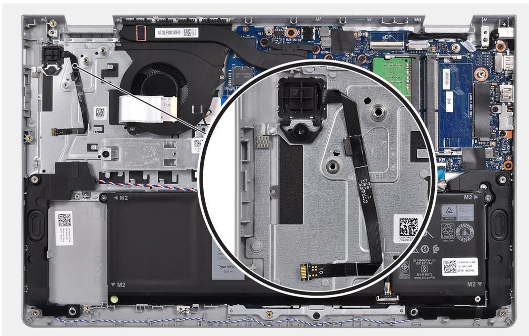
3. Re-adhere the tape to secure the fingerprint-reader FPC to the palm-rest and keyboard assembly.
