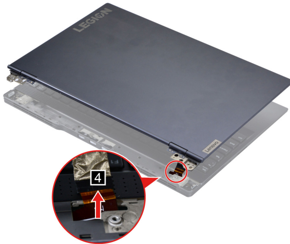
Figure 34. Take out the EDP cable and then remove the LCD module
