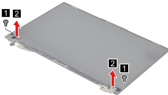
Figure 37. Remove two screws and remove the hinge caps
