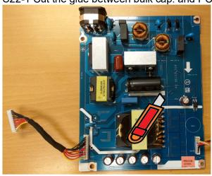
S22-2 Ensure cutting path within the glue, don't touch bulk cap. or PCB
