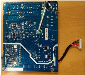
S22-4 Lift the bulk cap. up and away from the PCB
