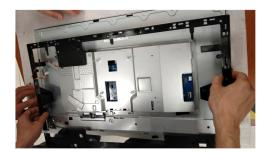
Tear off an adhesive tape from backlight wire and pull out backlight wire from Panel
