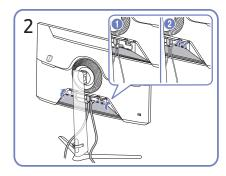
Arrange the cables against the bend tendency of the cables and pull the cables out of the COVER-REAR SUB grooves.
