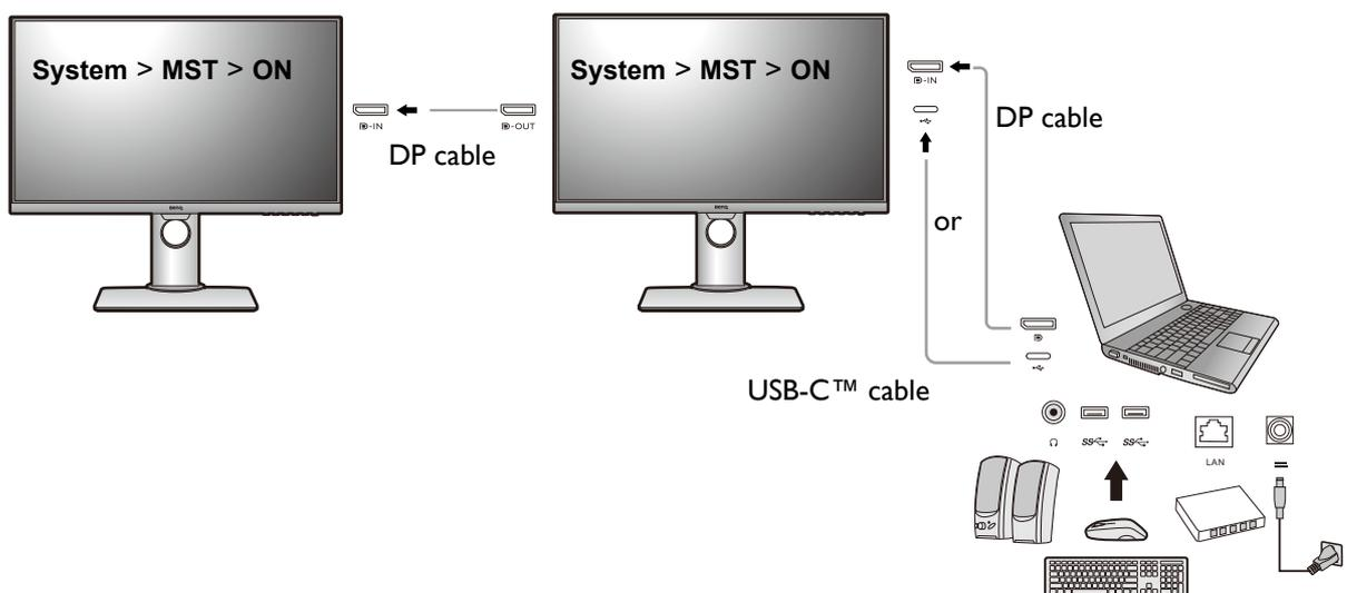
1. Connect your laptop to the USB-C™ / DP port on the monitor using a USB-C™ / DP cable. Select **Yes** to enable USB-C™ power delivery in monitor standby mode if you are prompted to. The USB-C™ port supplies power to the laptop then even when the monitor is in standby mode.
