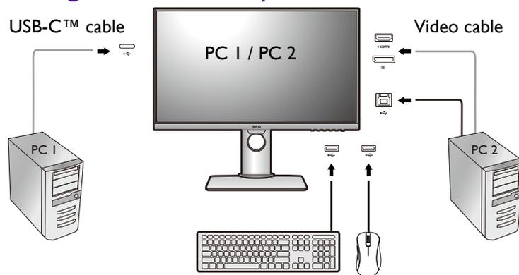
1. Establish cable connection as instructed in [Connect the PC video cable. on page 15](#).
