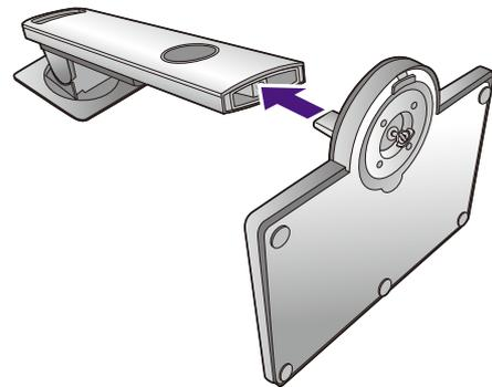
Tighten the thumbscrew on the bottom of the monitor base as illustrated.
