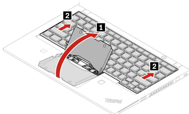
6. Pivot the keyboard slightly upward as shown by arrow **1**. Then, turn over the keyboard as shown by arrow **2**.
