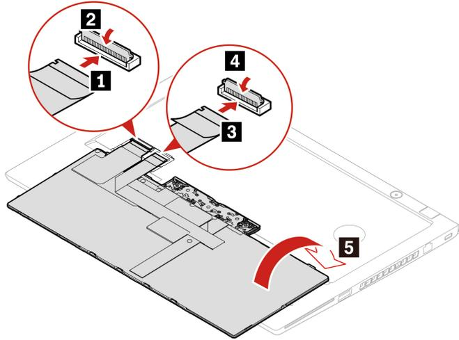
2. Insert the keyboard into the keyboard bezel as shown. Ensure that the top edge of the keyboard (the edge that is close to the display) is under the keyboard bezel.
