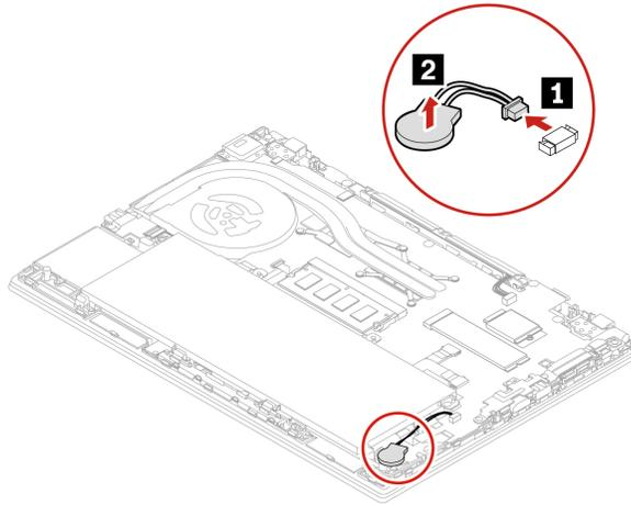
**Note:** After installation, reset the system date and time in the UEFI BIOS menu. See “Set the system date and time” on page 37.
