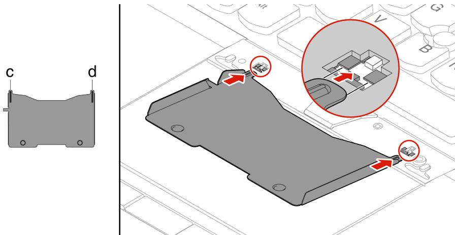
5. Pivot the tool in the direction as shown to release the keyboard **1**. Push the keyboard in the direction as shown by arrows **2** to release the latches from the keyboard bezel.
