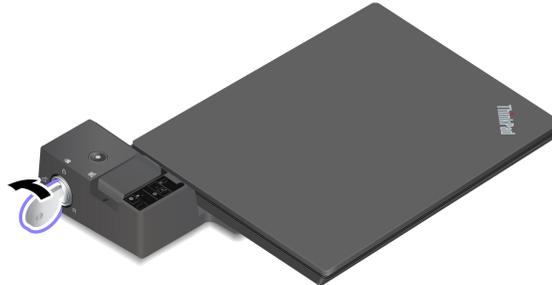
2. Slide the latch in the direction as shown **1** to release the computer, and then grasp both sides of the computer to remove it **2**.
