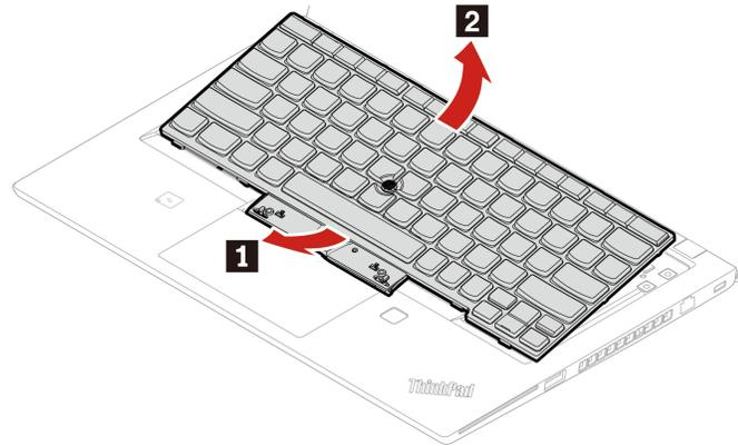
7. Put the keyboard on the palm rest as shown and detach the connectors. Then, remove the keyboard.
