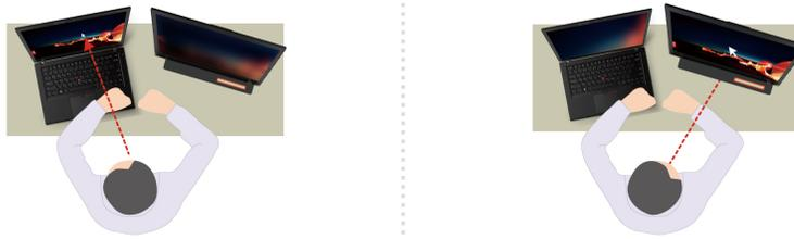
**Note:** Snap Window and Smart Pointer only work when your computer is connected to external displays. Ensure that external displays are placed at the same height of your computer.
