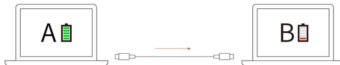
**Note:** The remaining battery power of computer A should be at least 30% and be 3% higher than that of computer B.
