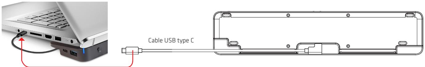
1. Please connect the black USB type C cable clicked onto the Dock and connect, the angled connector, to the Dock at that side of the Dock, connect the other side of that cable to the USB Type C port of your NoteBook/Host system.
