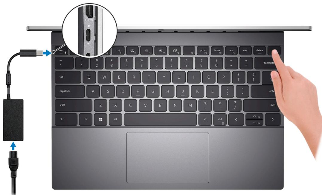
**NOTE:** The battery may go into power-saving mode during shipment to conserve charge on the battery. Ensure that the power adapter is connected to your computer when it is turned on for the first time.
