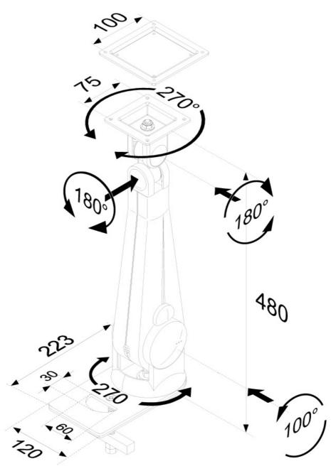
Neomounts Measuring unit: mm
