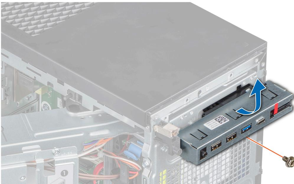
**Figure 52. Removal of the control panel**
