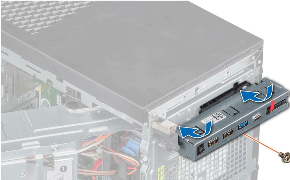
**Figure 53. Installing the control panel**
