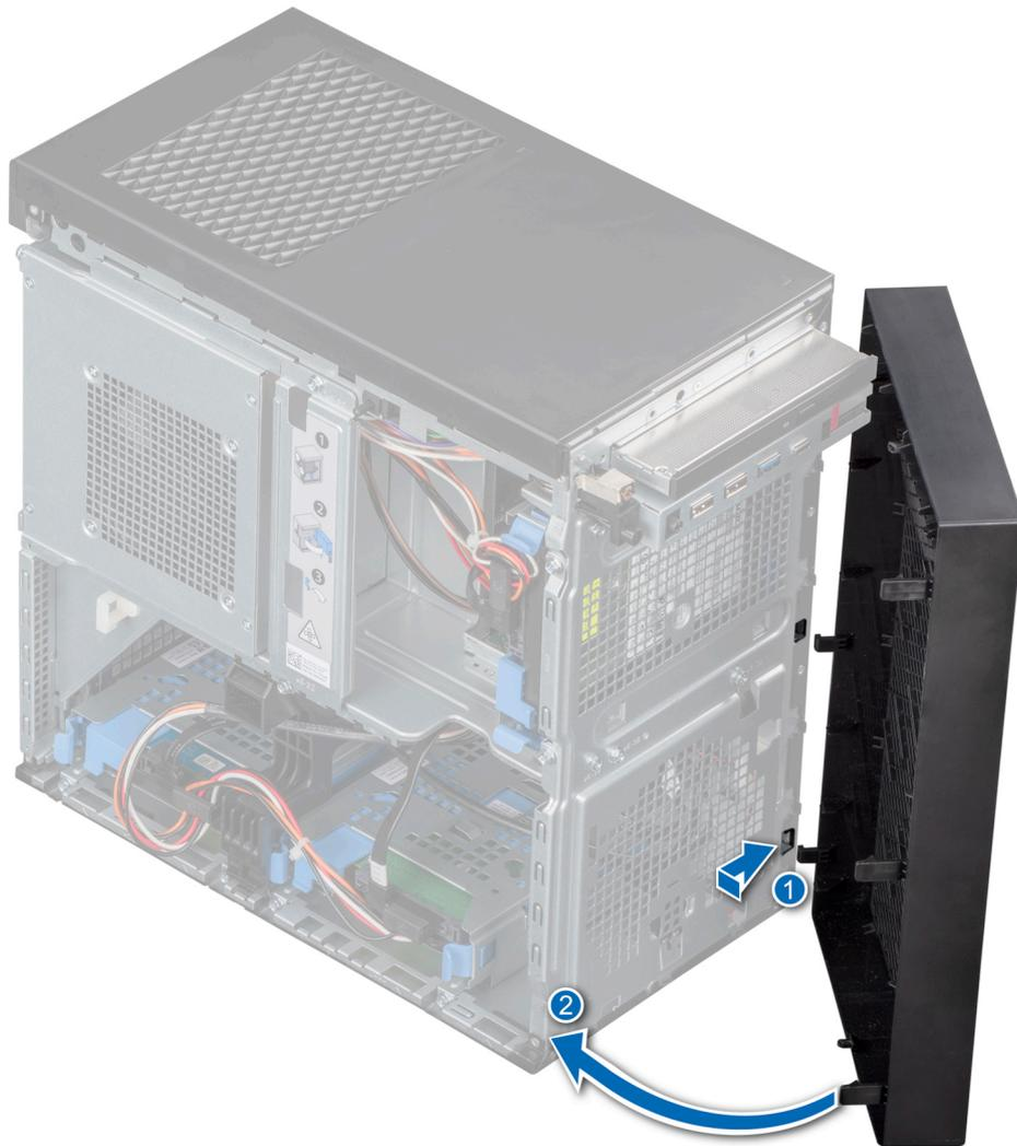
Figure 13. Installing the front bezel
