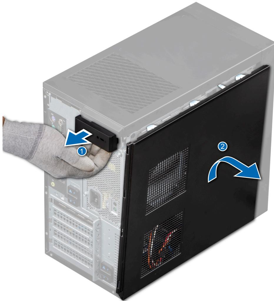
Figure 10. Removing system cover
