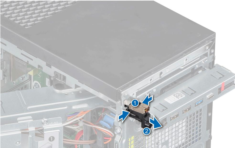
**Figure 54. Removing the power button module**
