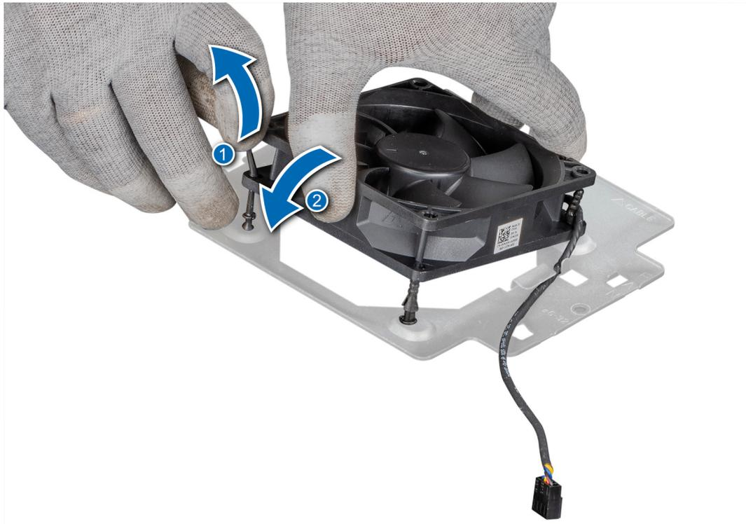
**Figure 39. Installing system fan**
