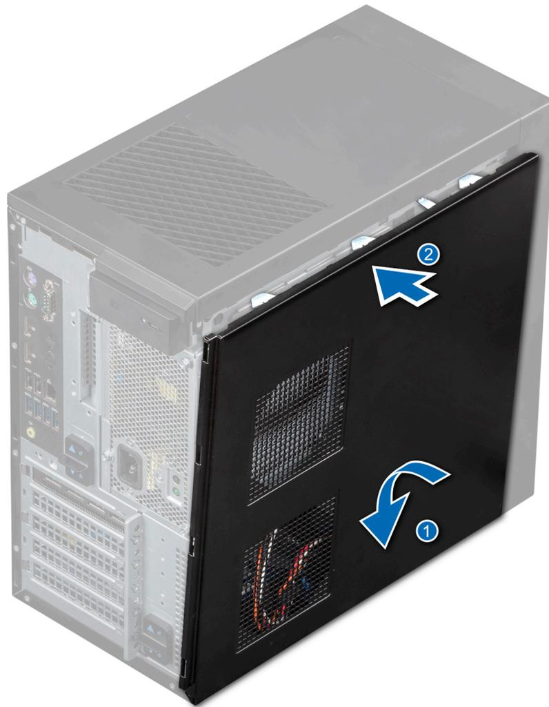
Figure 11. Installing the system cover
