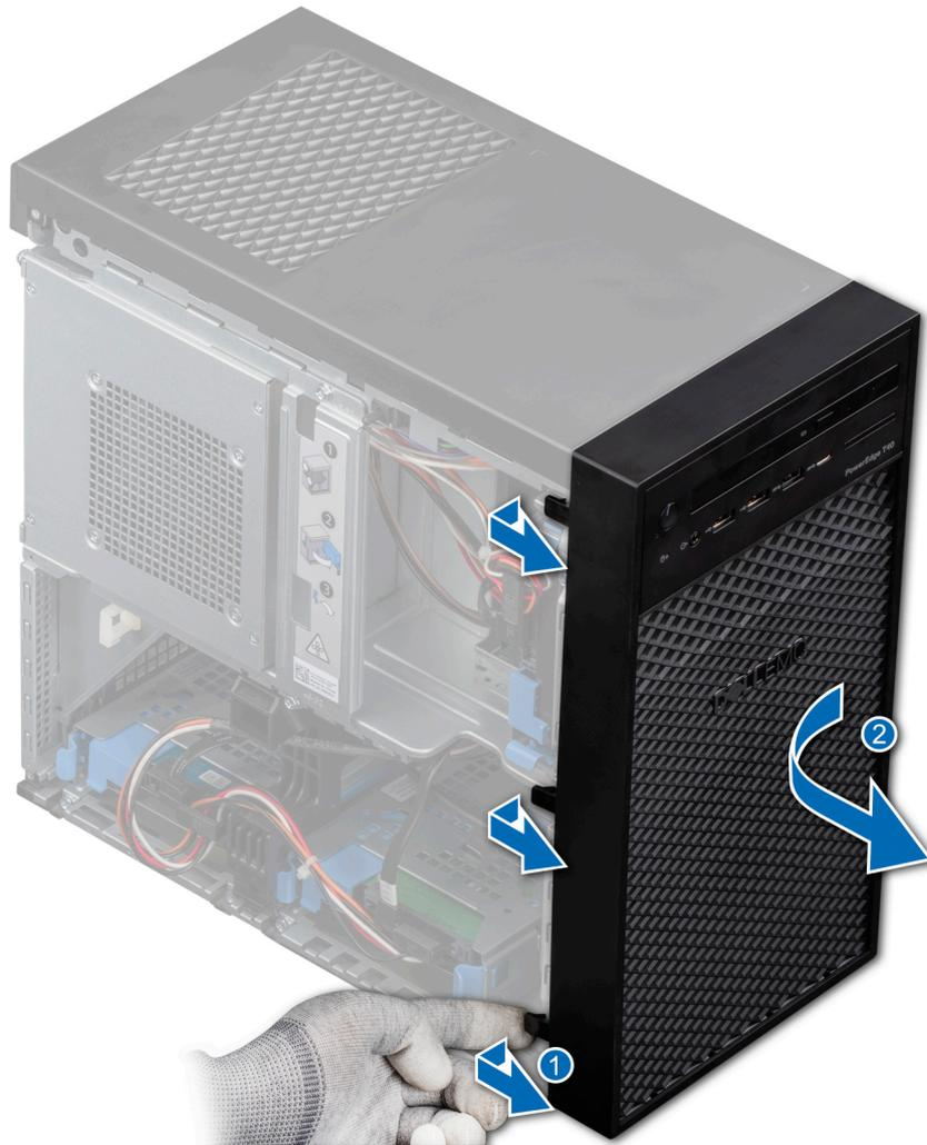
Figure 12. Removing the front bezel
