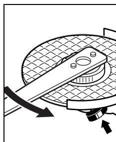
A properly attached, undamaged quick-clamping nut can be loosened by hand when turning the knurled ring in an anticlockwise direction.
