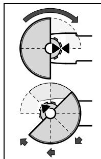
Place the protection guard **12** onto the spindle collar as shown in the illustration. The triangle marks on the protection guard must correspond with the respective marks on the gear case.
