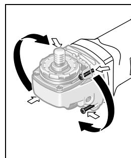
The machine head can be rotated with respect to the machine housing in 90° steps. In this manner, the On/Off switch can be brought into a more convenient position for special working situations, e. g., for cutting operations using the cutting guide with dust extraction protection guard 21 or for left-handed persons.
