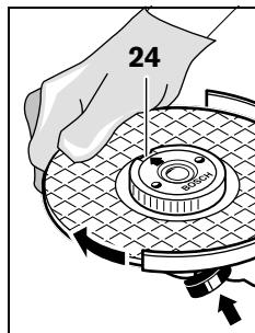
Lock the grinder spindle with the spindle lock button 2. To tighten the quick-clamping nut, firmly turn the grinding disc in clockwise direction.
