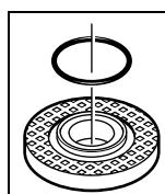
A plastic part (O-ring) is fitted around the centring collar of mounting flange **8**. **If the O-ring is missing or damaged, the mounting flange 8 must be replaced before resuming operation.**
