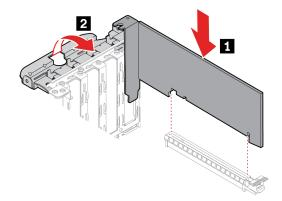
**Note:** During the installation, ensure that you align the PCI-Express card to the slot and press down until the latch is fully engaged with a click.
