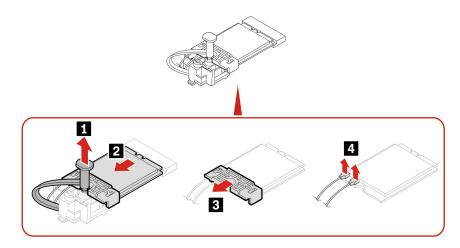
**Note:** During installation, ensure that you connect the gray cable to the connector labeled AUX on the card, and the black cable to the connector labeled MAIN.
