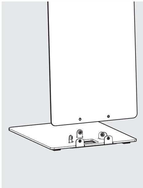
**1** Locate the Mounting Arm onto the Freestanding Base.
