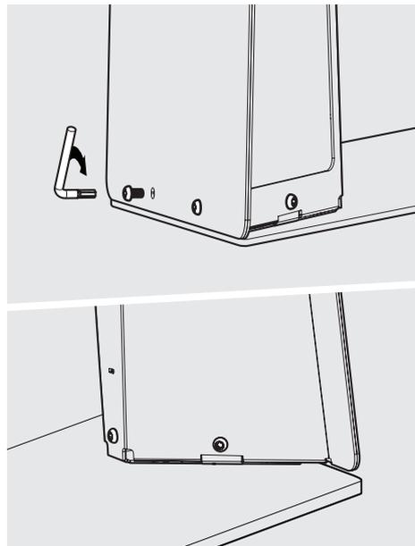
**2** Secure the Mounting Arm to the Mount Bracket, with 5x M6x10mm screws.
