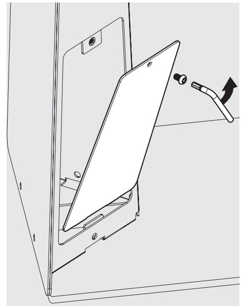
**3** Remove the Mounting Arm Access Panel. Safely store this aside for use later.
