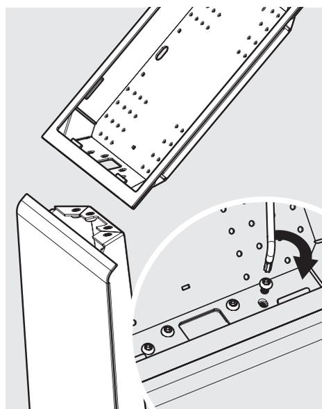
**5** Locate and secure the Case Back to the Mounting Arm, with 4x M6x10mm screws. Ensure good Case alignment.
