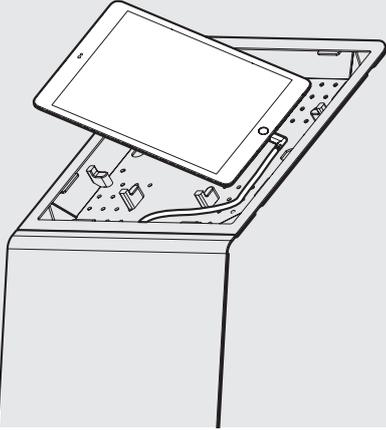
**7** Install the tablet and the tablet power cable.
