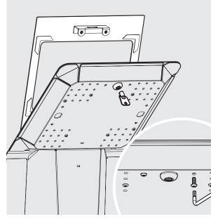
Locate and lock the Faceplate onto the Case Back. For additional security, install 2x M4x10mm screws to retain the Faceplate.
