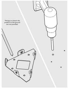
Mark your mounting surface, then drill (as appropriate to your chosen fixing method).
