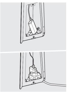
11 Connect the tablet to a power source.
