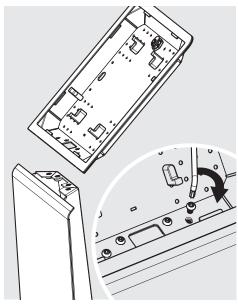
Locate and secure the Case Back to the Mounting Arm, with 4x M6x10mm screws. Ensure good Case alignment.
