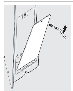
Remove the Access Panel from the Mounting Arm. Store all parts safely aside for use later.
