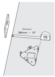
Position the Mount Bracket on the ground where the stand is to be located.
