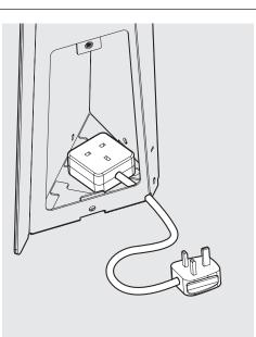
If using a hard-wired power supply, feed the cable into the Mounting
