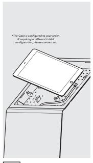
lnstall the tablet and the tablet power cable.
