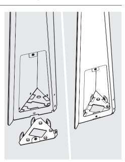
6 Locate the Mounting Arm onto the Mount Bracket as shown.
