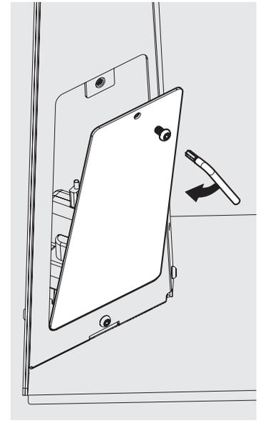
**9** Locate and secure the Access Panel to the Mounting Arm.
