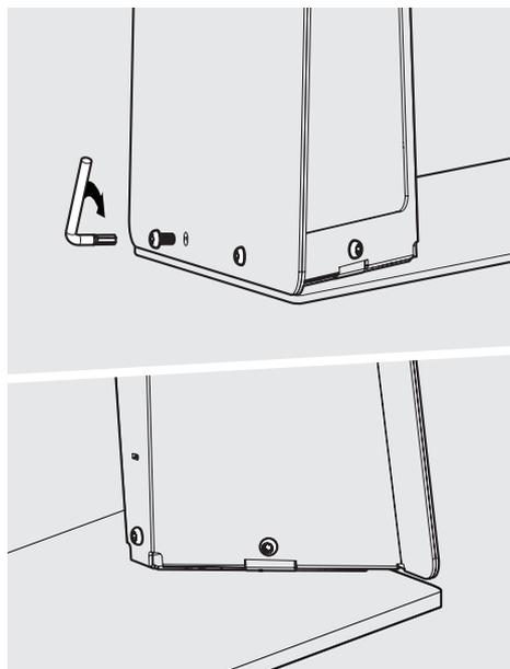
**2** Secure the Mounting Arm to the Mount Bracket, with 5x M6x10mm screws.
