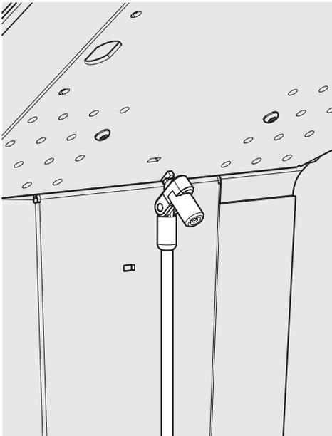
**10** For additional security, the stand has multiple Kensington Security Slots. Where required, install the cable.
