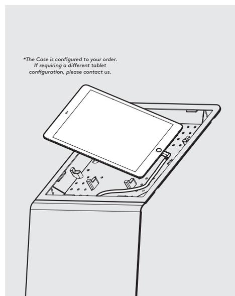
**6** Install the tablet and the tablet power cable.
