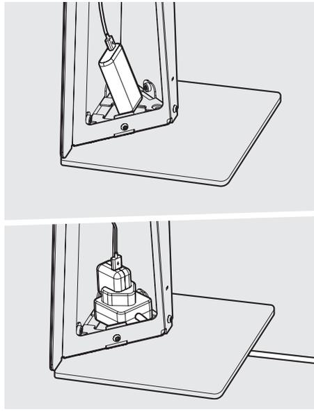
**8** Connect the tablet cable to a power source.
