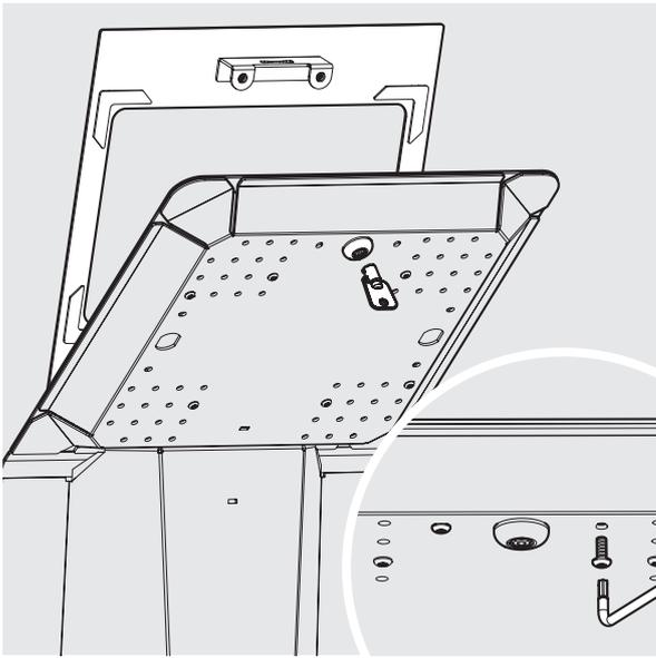
**7** Locate and lock the Faceplate onto the Case Back. For additional security, install 2x M4x10mm screws to retain the Faceplate.
