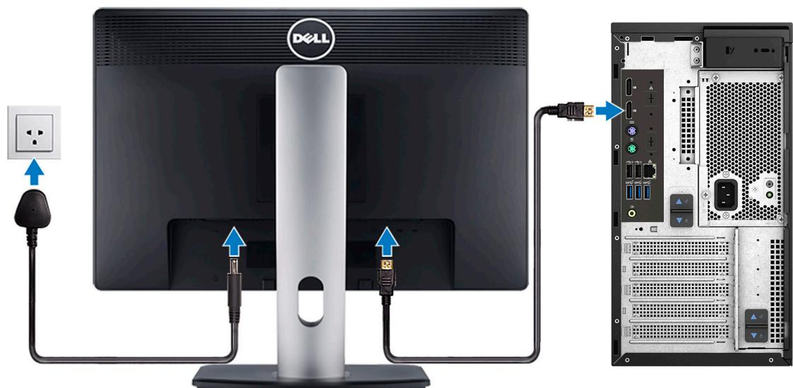
***(i) NOTE:*** If you ordered your computer with a discrete graphics card, connect the display cable to the discrete graphics card connectors.
