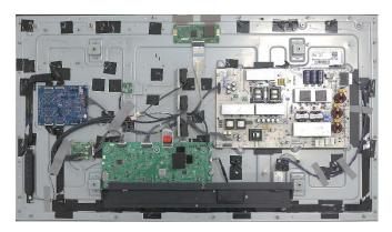
LCD module(together with their casing) is only left after all other parts like electronic units and casing have been removed.
