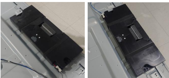
Remove the speaker units. (L/R)
