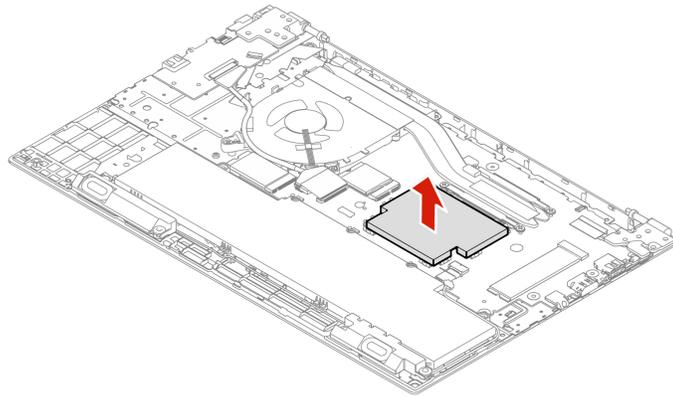
6. Open the latches on both sides of the memory module slot at the same time **1**, and then remove the memory module **2**.
