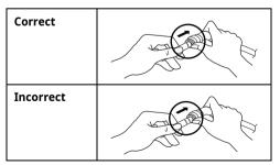
• If the water tube end is damaged, it should be trimmed to ensure it does not leak when refitted.
