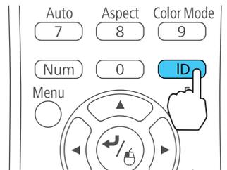
5. Press the **ID** button on the remote control to check if the ID-setting process worked. You see a message displayed by the projector.
