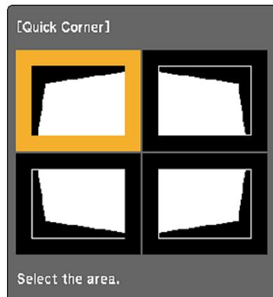
**Note:** To reset your adjustments, press and hold the **Esc** button for at least 2 seconds to display a reset screen. Then select **Yes**.
