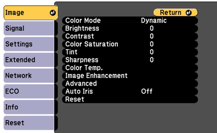
2. Press the up or down arrow button to move through the menus listed on the left. The settings for each menu are displayed on the right.
