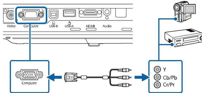
3. Tighten the screws on the VGA connector.
