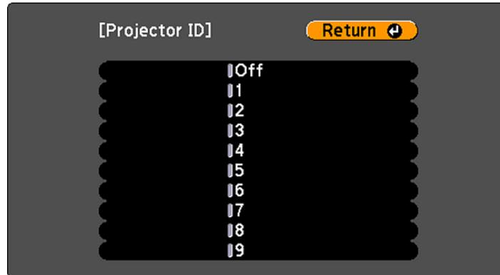
4. Press the arrow buttons on the remote control to select the identification number you want to use for the projector. Then press **Enter**.
