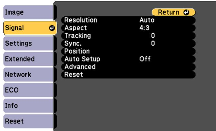
**Note:** You can restore the default settings of the **Position**, **Tracking**, and **Sync** settings by pressing the **Auto** button on the remote control.
