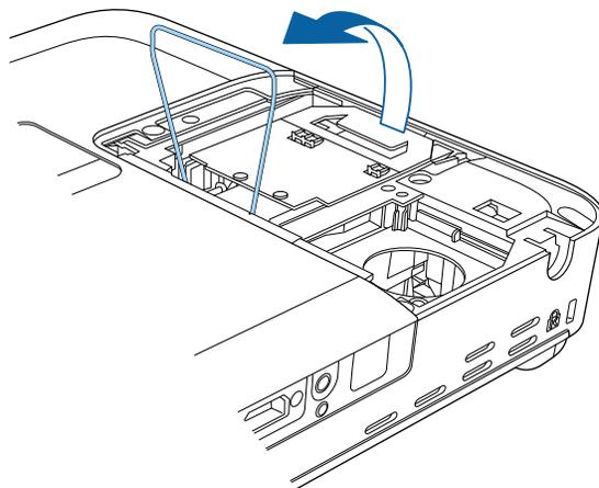
6. Lift up the lamp handle and gently pull the lamp out of the projector.
