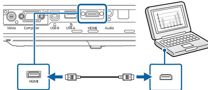
**Note:** The projector converts the digital audio signal sent from your computer into a mono analog signal for the internal speaker. If you have problems hearing audio through the HDMI connection, connect one end of an optional 3.5 mm stereo mini-jack audio cable to the projector's **Audio** port and the other end to your computer's audio out port. Then select the audio port you connected to as the **HDMI Audio Output** setting in the Extended menu.
