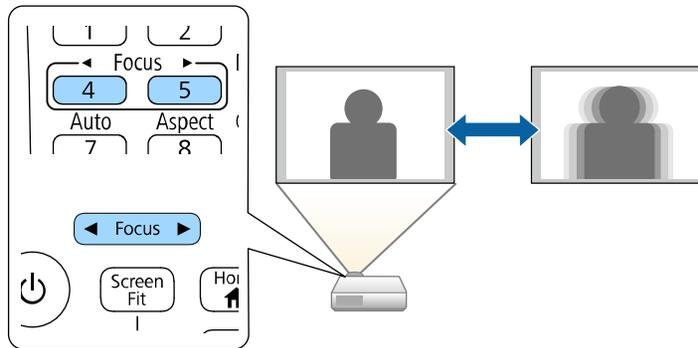
3. Press and hold the arrow buttons on the projector's control panel or remote control to adjust the focus.
