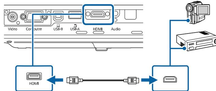
**Note:** The projector converts the digital audio signal sent from your video source into a mono analog signal for the internal speaker.
