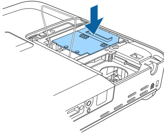
**Caution:** Do not touch any glass on the lamp assembly to avoid premature lamp failure.
