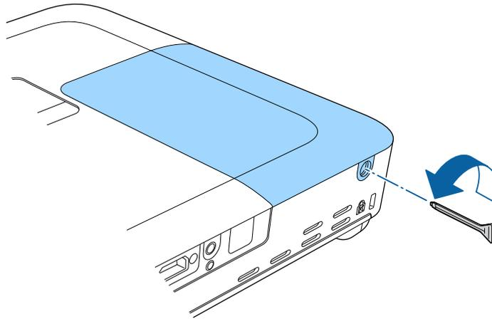
**Warning:** If the lamp is broken, glass fragments may be loose inside the lamp chamber. Be careful removing any broken glass to avoid injury.
