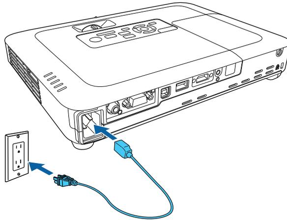
3. Plug the power cord into an electrical outlet.
