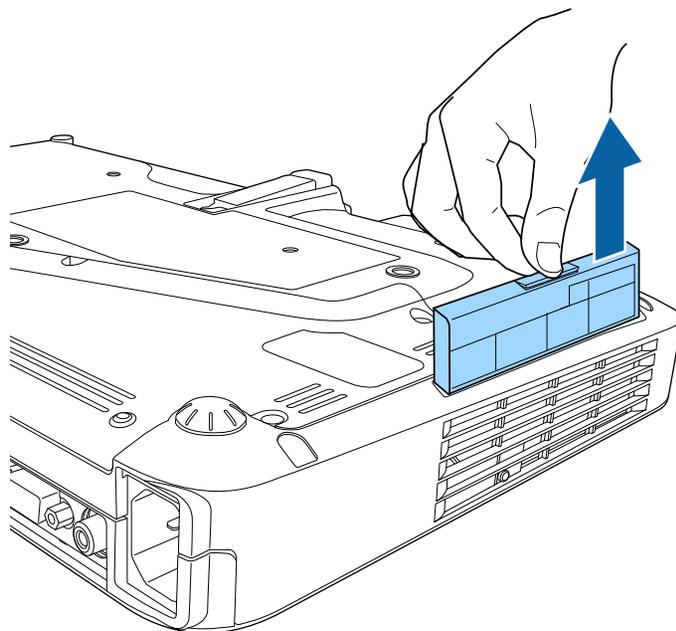
**Note:** Air filters contain polycarbonate, ABS resin, and polyurethane foam. Dispose of used air filters according to local regulations.
