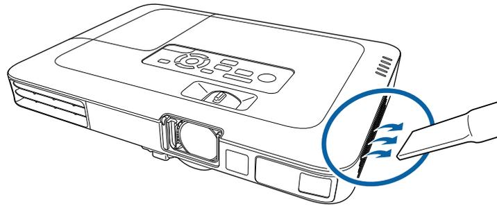
**Note:** You can remove the air filter so you can clean both sides of it. Do not rinse the air filter in water, or use any detergent or solvent to clean it.
