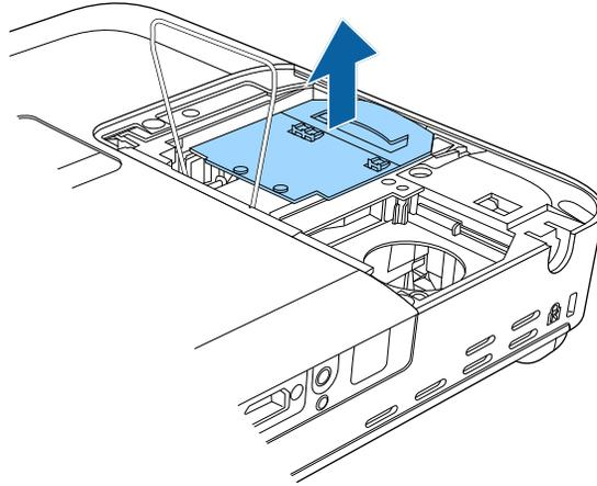
**Caution:** Lift the lamp handle carefully to avoid damaging the handle as you pull out the lamp.
