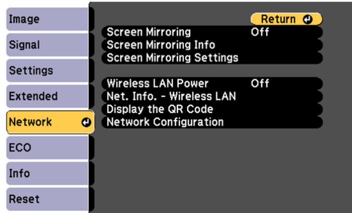
4. Make sure the **Wireless LAN Power** setting is set to **On**.
