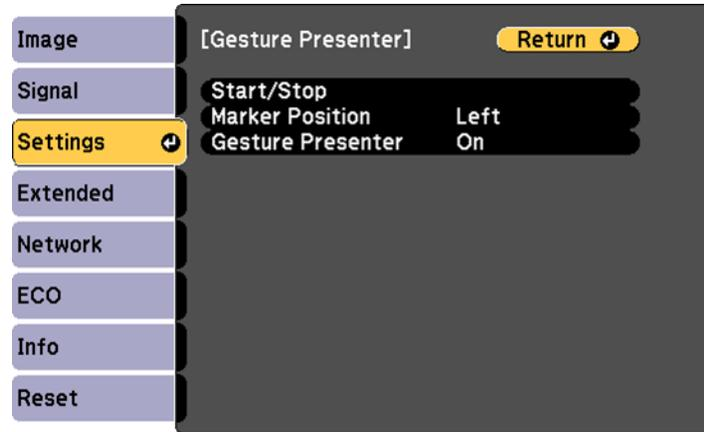
**Note:** You can also display the Gesture Presenter settings by pressing and holding down the **Screen Fit** button on the projector for three seconds.
