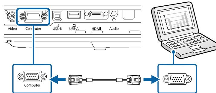
4. Tighten the screws on the VGA connector.
