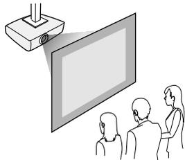
Wherever you set up the projector, make sure to position it squarely in front of the center of the screen, not at an angle, if possible.
