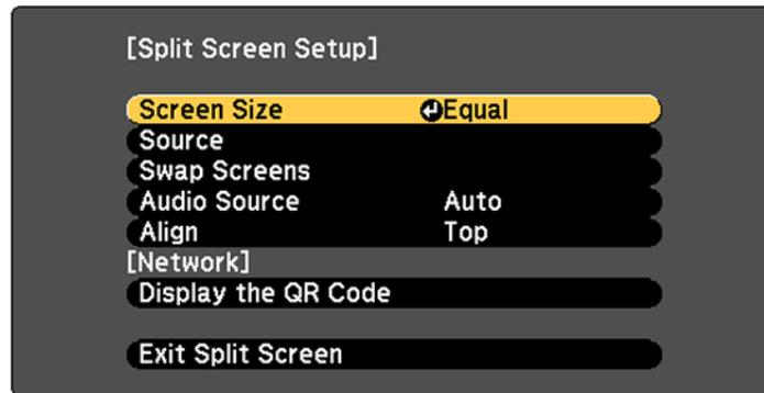
3. To select an input source for the other image, select the **Source** setting, press **Enter**, select the input source, select **Execute**, and press **Enter**. (You can also change image sources, if necessary.)
