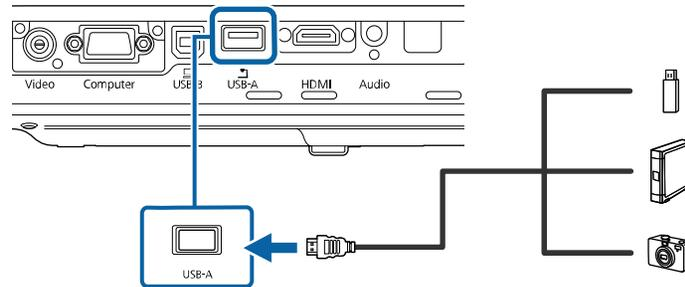
**Note:** Do not connect a USB hub or a USB cable longer than 10 feet (3 m), or the device may not operate correctly.
