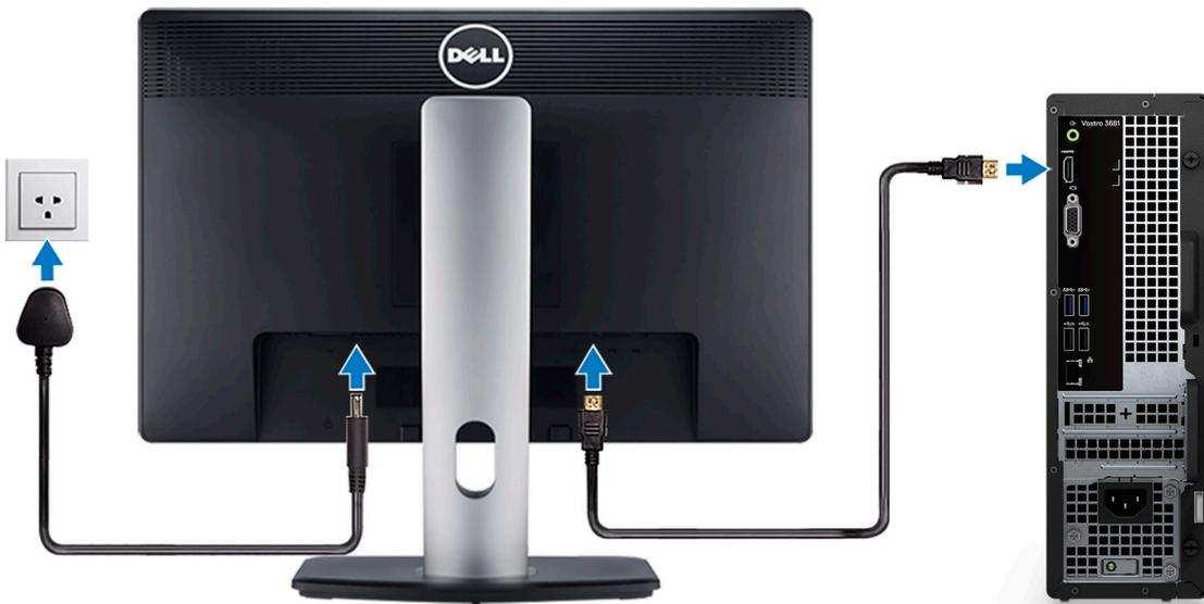
**NOTE:** If you ordered your computer with a discrete graphics card. Connect the display cable to the discrete graphics card connectors.
