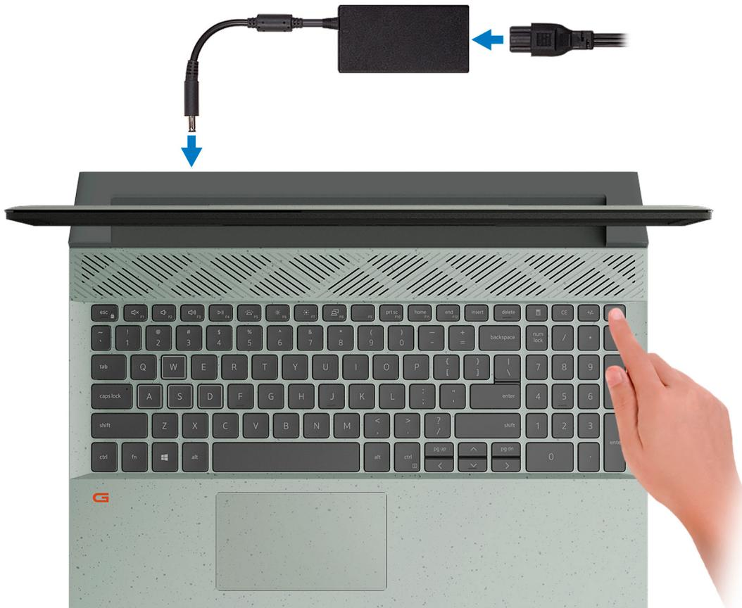
***(i)* NOTE:** To conserve battery power, the battery might enter power-saving mode. Connect the power adapter and press the power button to turn on the computer.
