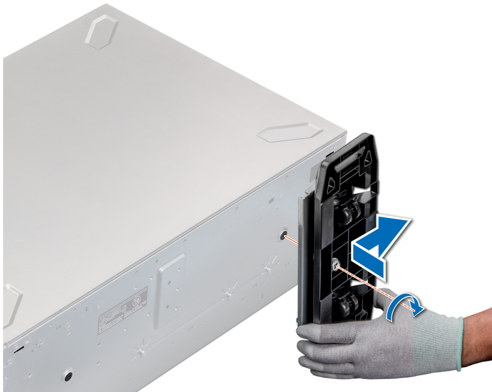
Figure 22. Installation des roulettes
