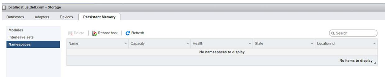
The screenshot shows the ESXi storage configuration page for NVDIMM namespaces. The left sidebar has 'Namespaces' selected. The main table is empty, displaying 'No namespaces to display'.
