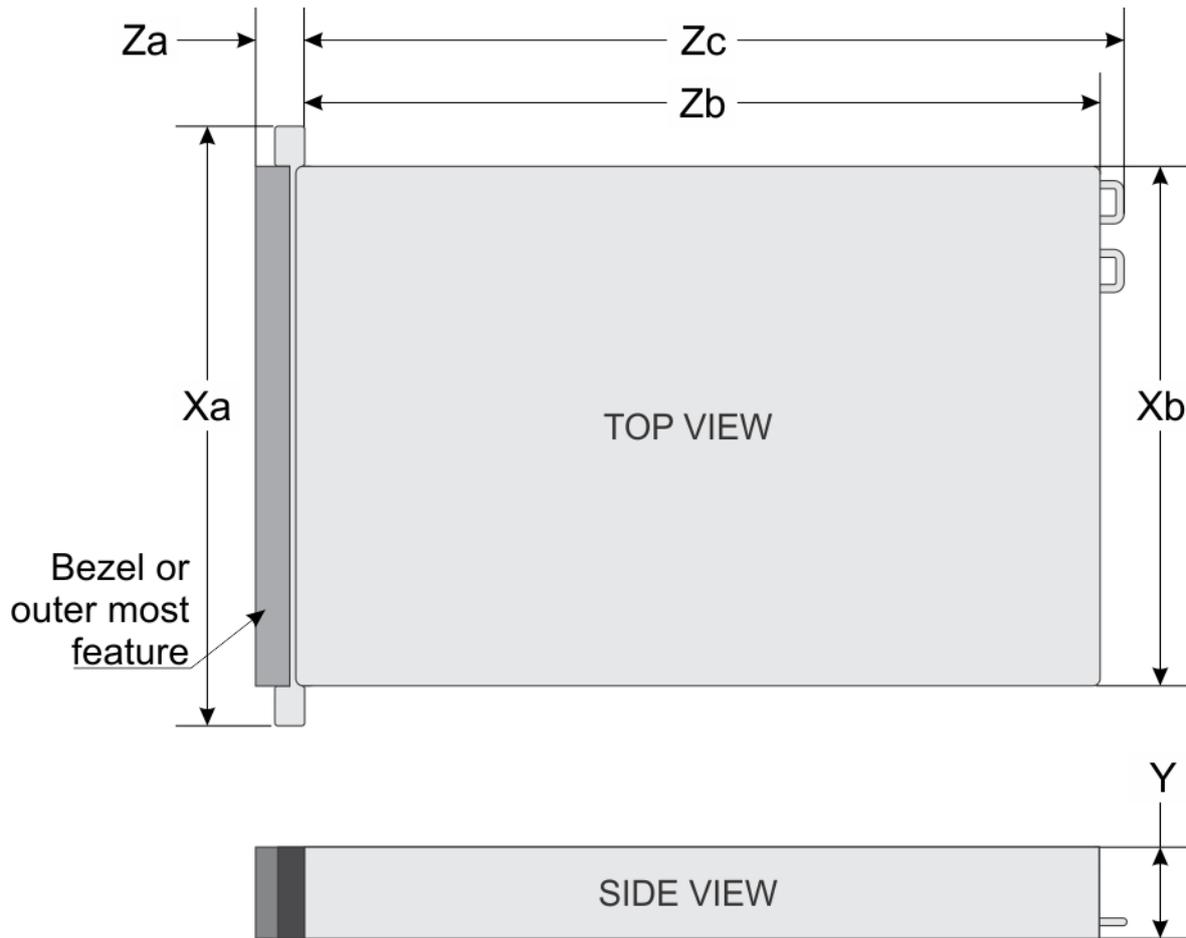
Figure 1. System dimensions of PowerEdge R740 system
