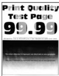
**Note:** Before solving the problem, print the Print Quality Test Pages. From the control panel, navigate to **Settings > Troubleshooting > Print Quality Test Pages**. For non-touch-screen printer models, press
