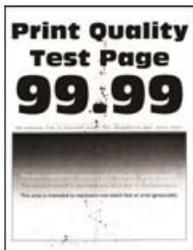
**Note:** Before solving the problem, print the Print Quality Test Pages. From the control panel, navigate to **Settings > Troubleshooting > Print Quality Test Pages**. For non-touch-screen printer models, press **OK** to navigate through the settings.
